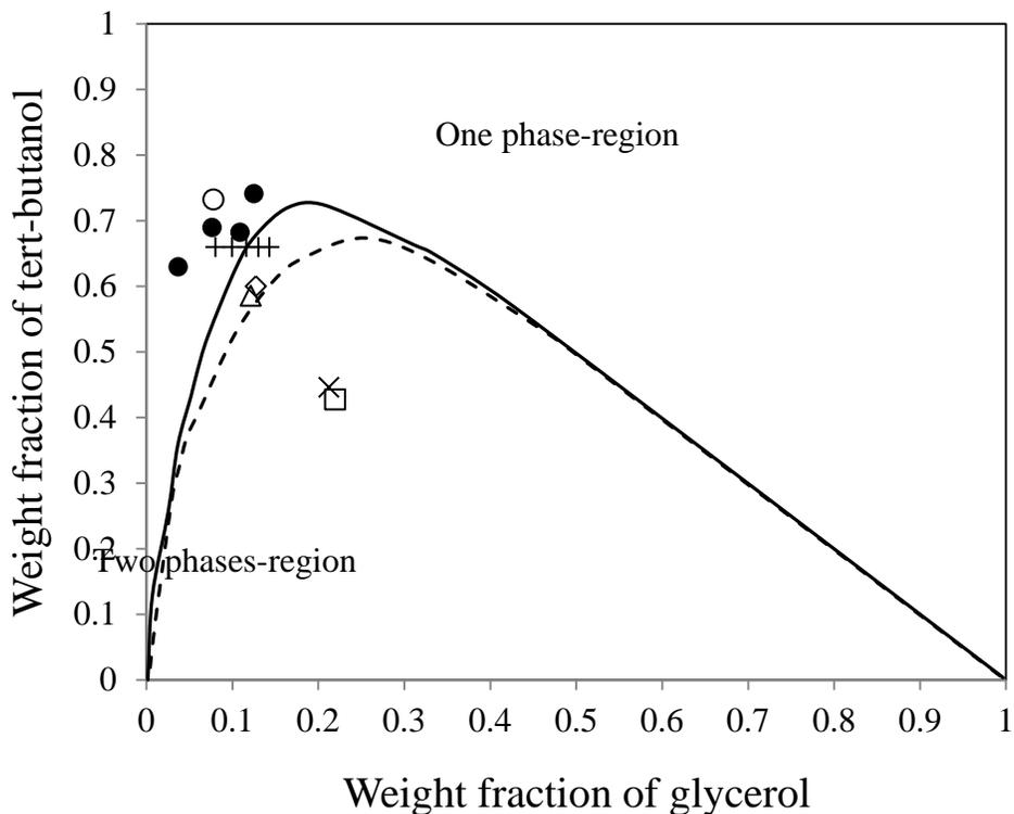
**Figure 5.** Binodal curve of the ternary system glycerol + fish oil + tert-butanol at 303.15 K (—) and 323.15 K (---). Initial composition of glycerolysis reaction in tert-butanol medium:  $\bullet$  this work,  $\circ$  Sunflower oil [8],  $\diamond$  Sunflower oil [20],  $\Delta$  Tuna oil [37],  $+$  Camellia oil [19],  $\square$  Olive oil [17],  $\times$  Olive oil [16].
