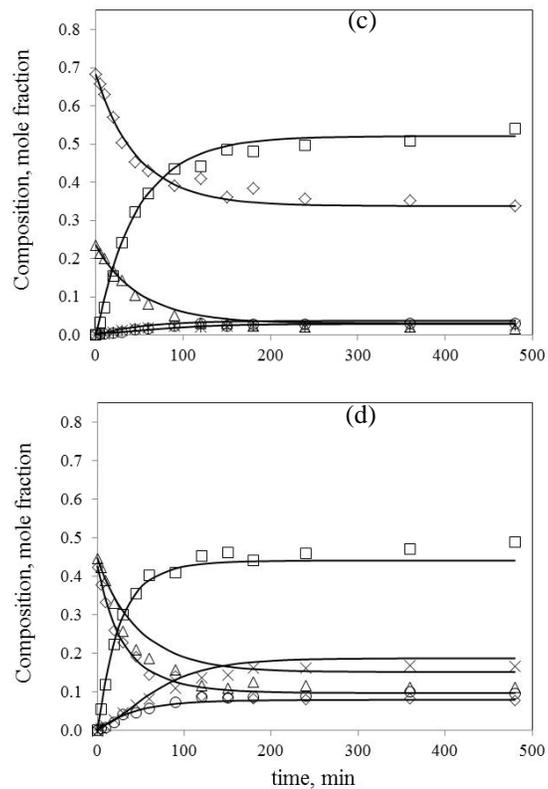
**Figure 3.** Time course of the glycerolysis reaction at different mole ratios (MR): (a) 9:1, (b) 5:1, (c) 3:1 (d) 1:1; 323 K, 10 wt % Lipozyme<sup>®</sup> 435 loading;  $\square$  MAG  $\circ$  FFA  $\Delta$  TAG  $\diamond$  glycerol  $\times$  DAG. Continuous lines are for the model in this work. Standard uncertainty  $u$  (mole fraction) = 0.02.
