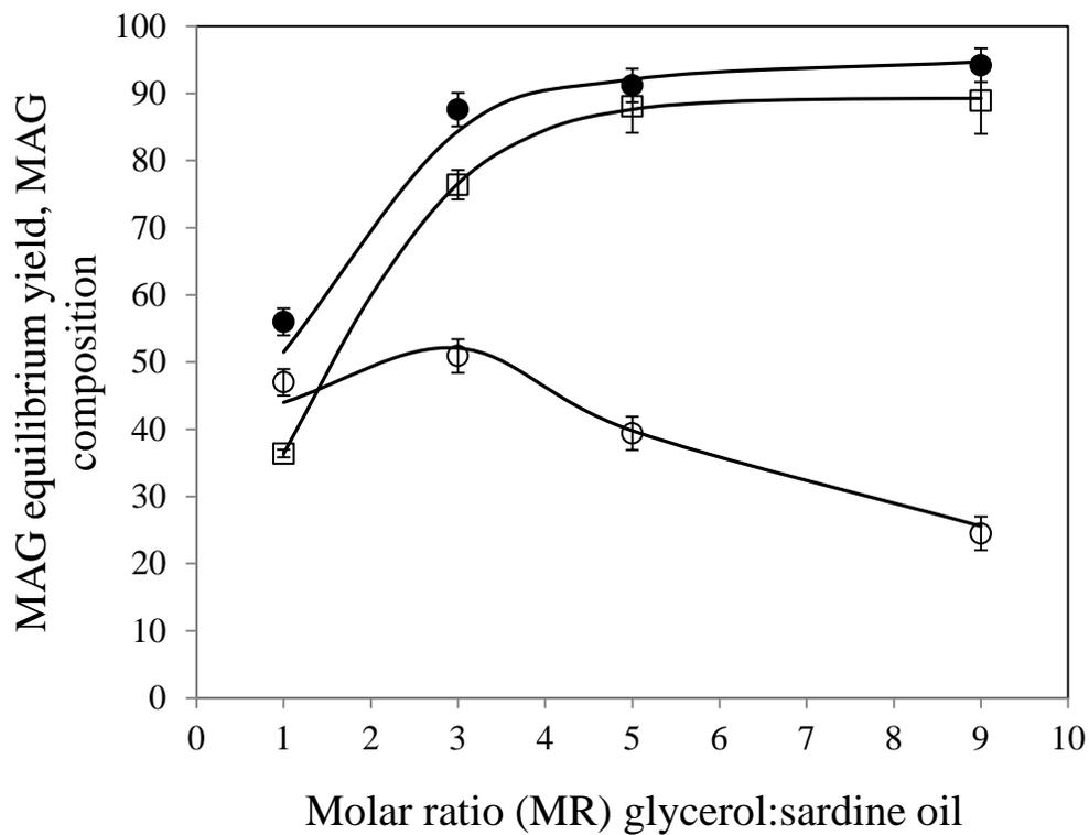
**Figure 4.** MAG equilibrium yield ( $\square$ ) as a function of initial mole ratio (MR) glycerol:oil. The continuous line is for Eq. 20. MAG composition as mole percentage on a solvent and glycerol free-basis ( $\bullet$ ) and on a solvent free-basis ( $\circ$ ). Continuous lines are the equilibrium composition obtained with the model in this work.
