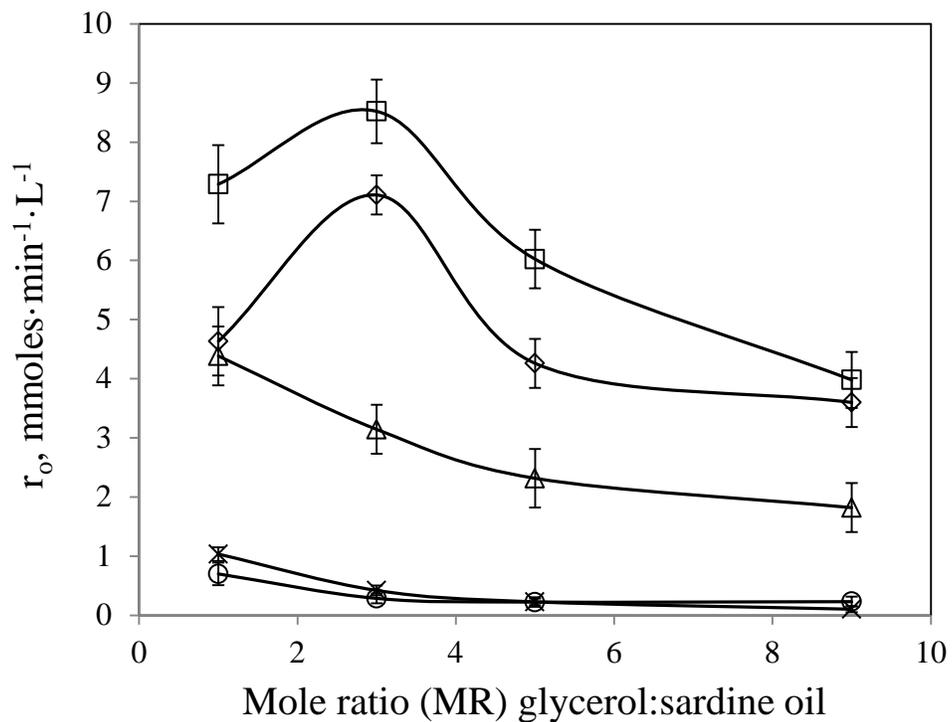
**Figure 6.** Initial reaction rate as a function of initial mole ratio glycerol:oil (323 K, 10 wt % Lipozyme<sup>®</sup> 435 loading):  $\square$  MAG  $\circ$  FFA  $\triangle$  TAG  $\diamond$  glycerol  $\times$  DAG.
