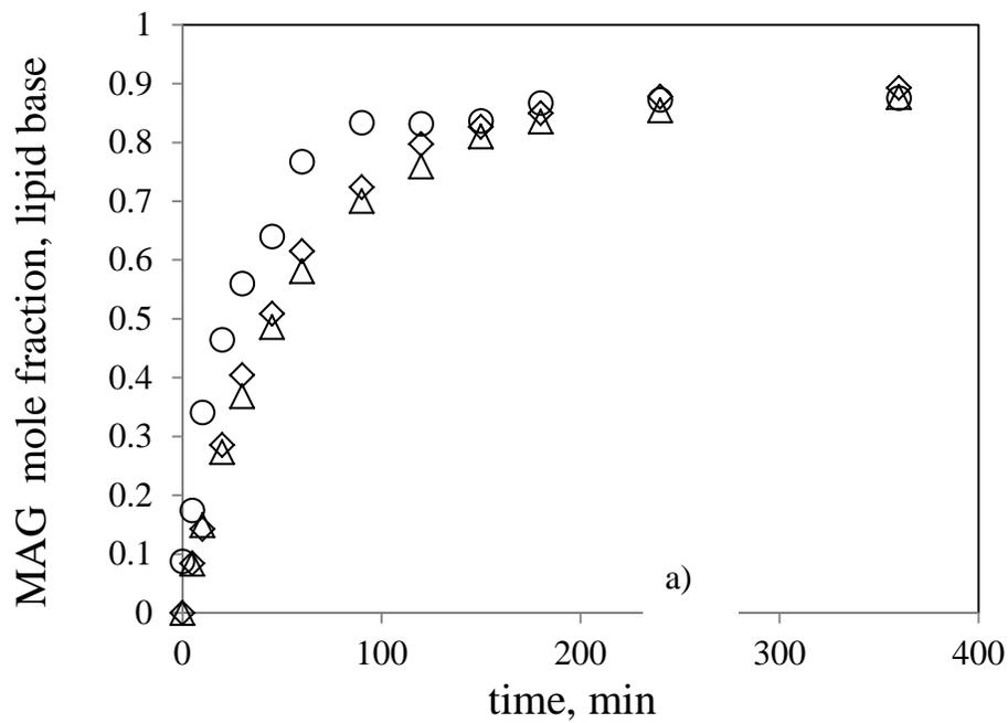
**Figure 2.** Effect of particle size (○)  $d_p < 400 \mu\text{m}$ ; (◇) unsieved lipase; (△)  $d_p > 400 \mu\text{m}$  on MAG formation reaction:  $T = 323 \text{ K}$ , 5 wt % Lipozyme<sup>®</sup> 435 loading,  $\text{MR} = 3:1$ . Standard uncertainty  $u$  (mole fraction) = 0.02.
