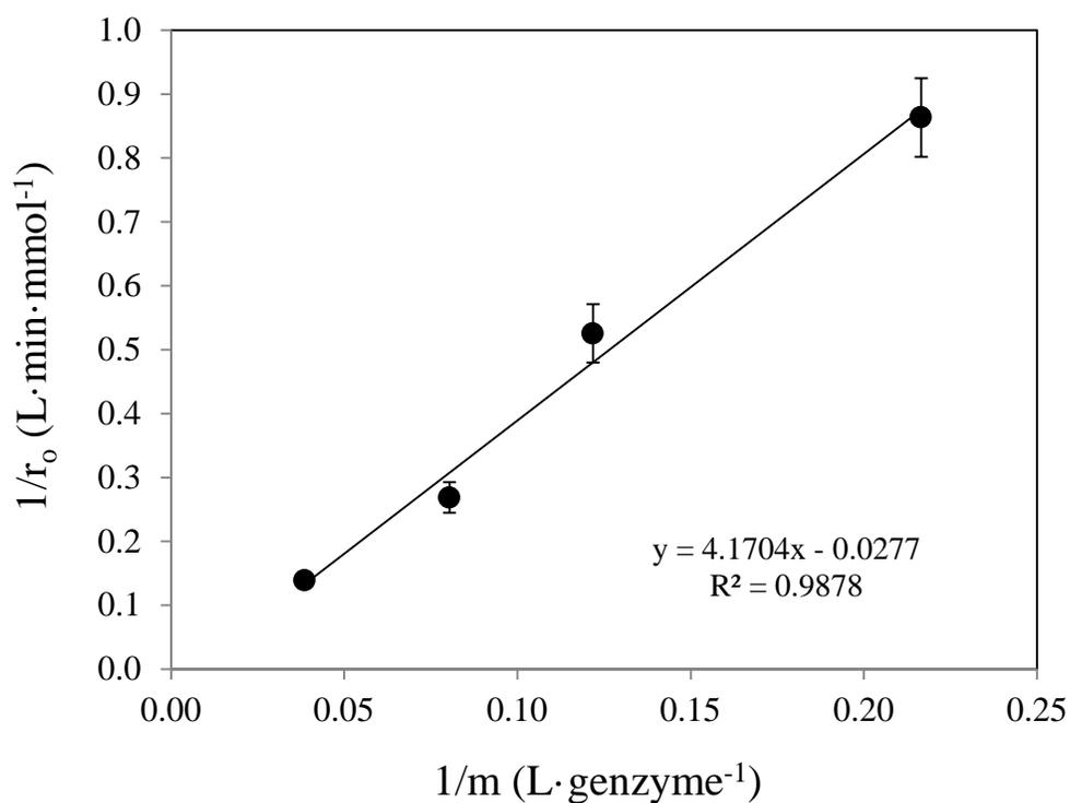
**Figure 1.** Effect of catalyst loading on initial reaction rate of MAG formation (T = 323 K, MR = 3:1).
