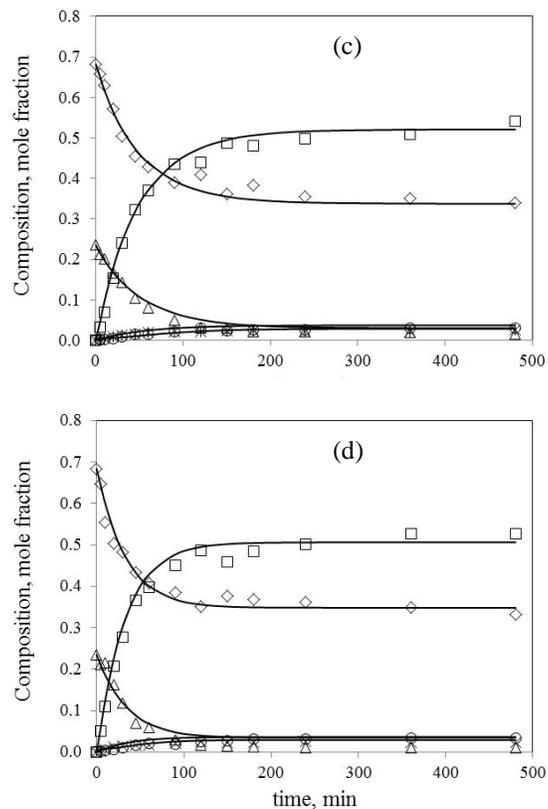
**Figure 7.** Time course for the glycerolysis reaction at different temperatures: ( a) 303 K, (b) 313 K, (c) 323 K, (d) 333 K; 10 wt % Lipozyme<sup>®</sup> 435 loading, MR =3:1; □ MAG ○ FFA △ TAG ◇ glycerol × DAG. Continuous lines are for the model in this work. Standard uncertainty  $u$  (mole fraction) = 0.02.
