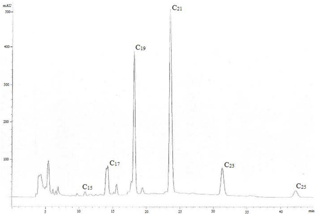
Figure 1. HPLC-DAD chromatogram of AR in wheat bran oil obtained in run R6
