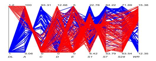
Figure 5. Parallel coordinates plot of the pareto-optimal solutions in section 3.2 with dosage level 1 % and without B component. *A-E* are for the percentage of these chemicals; *S*1 (Mpa) is the strength after one day, *S*7 (Mpa) after 7 days, and *S*28 (Mpa) after 28 days, *WR* (%) is water reduction.
