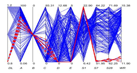
Figure 4. Parallel coordinates plot of the pareto-optimal solutions in section 3.2 only for dosage level 1 % (blue continuous lines) or 1.2 % (dotted red lines), and removing the coordinate for *B* (which is always 0%). *DL* is the dosage level, *A-E* are for the percentage of these chemicals; *S*1 (Mpa) is the strength after one day, *S*7 (Mpa) after 7 days, and *S*28 (Mpa) after 28 days, *WR* (%) is water reduction.
