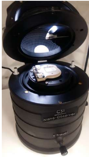
Fig. 5.8 CSI Nanoobserver AFM equipment.
