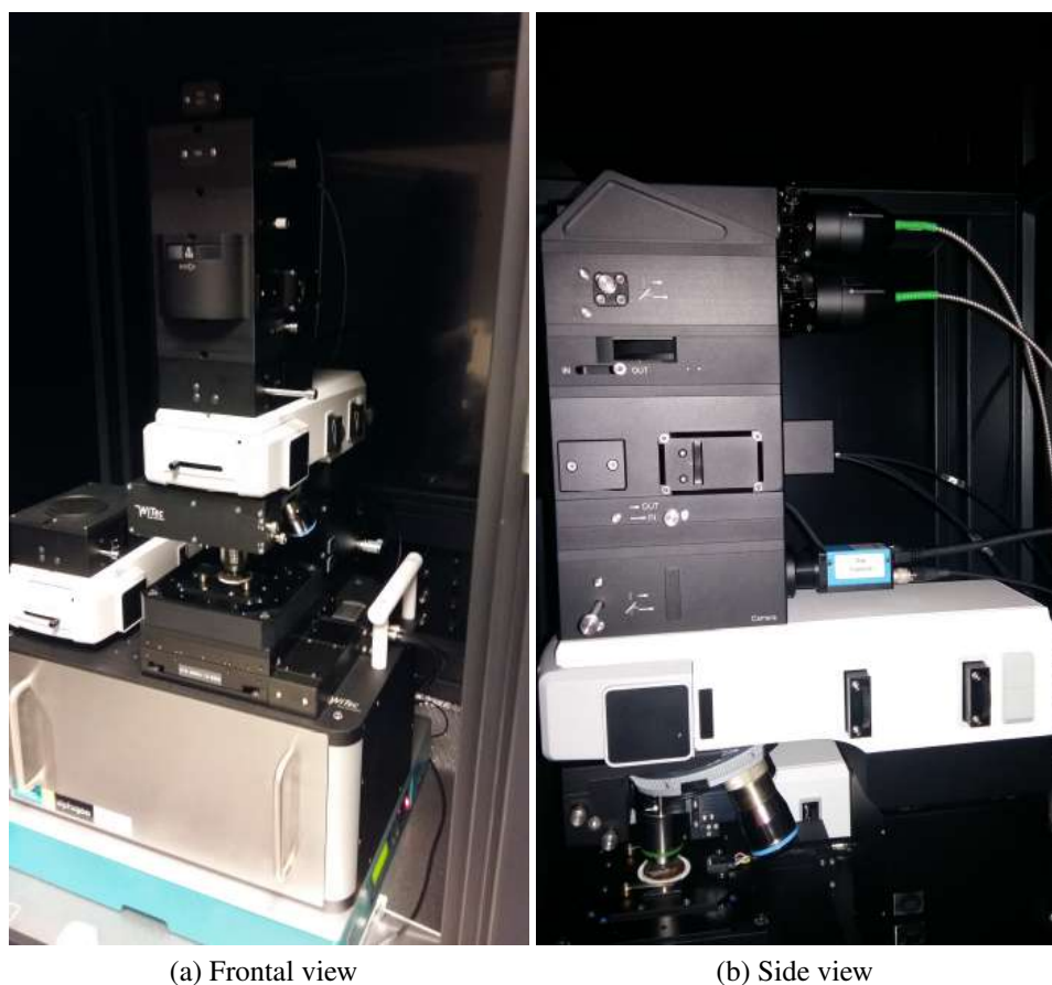
Fig. 5.4 Witec Confocal micro-Raman Alpha 300 R instrument.
