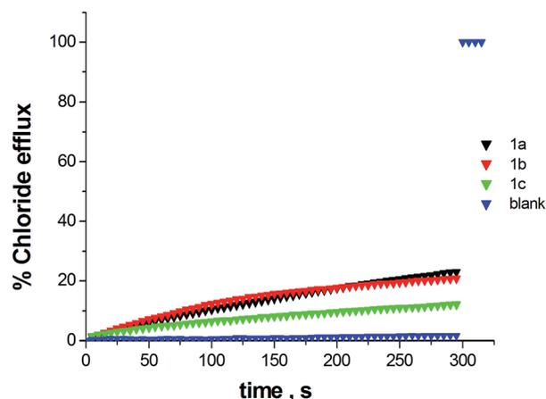
**Fig. 8** Chloride efflux promoted by compounds **1a–c** (75  $\mu\text{M}$ , 15% mol carrier to lipid concentration) in unilamellar POPC vesicles. Vesicles loaded with 450 mM NaCl buffered at pH 7.2 with 20 mM phosphate dispersed in 150 mM  $\text{Na}_2\text{SO}_4$  buffered at pH 7.2. Each trace represents the average of at least different three trials.
