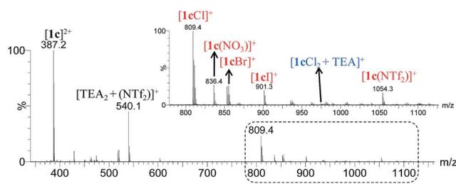
**Fig. 4** Competitive ESI mass spectrum of an equimolar mixture of **[1c](NTf<sub>2</sub>)<sub>2</sub>** and TEAX (X =  $\text{Cl}^-$ ,  $\text{Br}^-$ ,  $\text{I}^-$  and  $\text{NO}_3^-$ ) in MeCN. The inset shows the expanded region in the  $m/z$  750–1150 range illustrating the ion abundances of the species **[1c X]<sup>+</sup>**.
