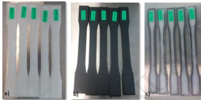
Figure 2. 3D Printed Specimens for a) Nylon b) Onyx and c) CFR composites.
