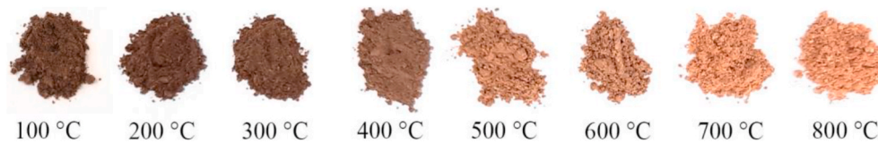
Fig. 7. Color change after controlled burning of sediment from SU XI at different temperatures for 1 h. (For interpretation of the references to color in this figure legend, the reader is referred to the Web version of this article.)
