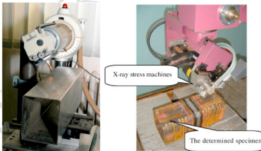
Fig. 11. X-ray diffraction apparatus for the residual stress determination in cold-rolled stainless steel hollow sections. Left picture extracted from Jandera et al. (2008) [144]; right picture from Tong et al. (2012) [142].
