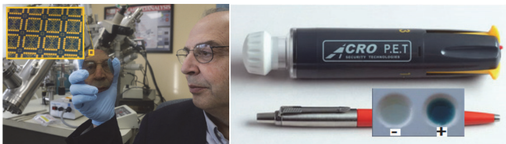
Figure 4. Novel devices to detect TATP. Left) Small footprint of thin film microheaters. Right) ACRO-P.E.T. – a simple to use pen like device.
