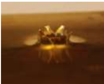
Figure 6.30.- Petalling fracture mode.
