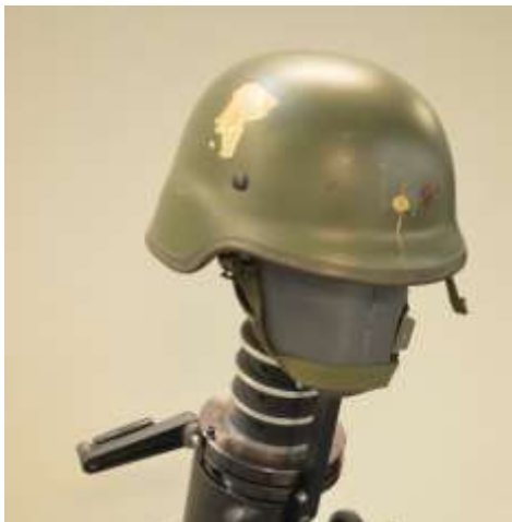
Figure 7.6.- Helmet after pistol ammunition impact.
