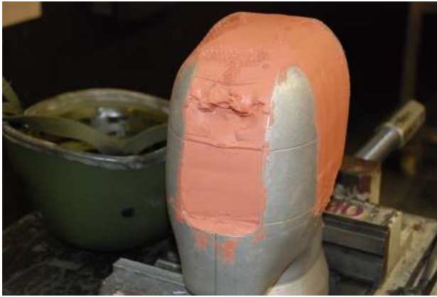
Figure 5.1.- US Army clay head after a 9 x 19 mm ballistic impact protected by the helmet in the frontal area.
