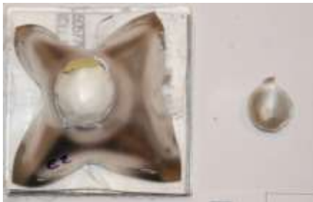
Figure 6.32.- Hertzian fracture in the back face of a sample.
