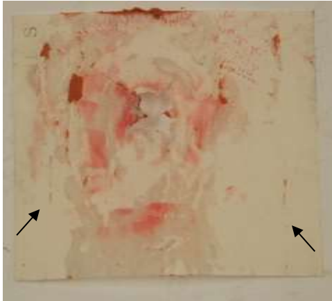
Figure 4.13.- Prescale film after the test (arrows point the petal marks).
