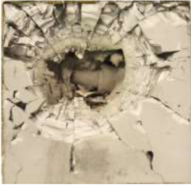
Figure 6.14.- 4 mm thickness SiC postmortem tile with the tumbled core.
