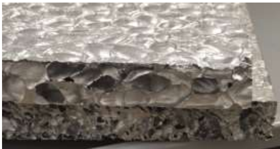
Figure 7.1.- Aluminium foams, 5 % (top) and 15 % (bottom) nominal aluminium density.
