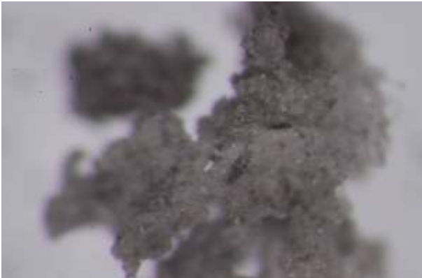
Figure 3.8.- Melted fibres retrieved from the impact point in UHMWPE composite.
