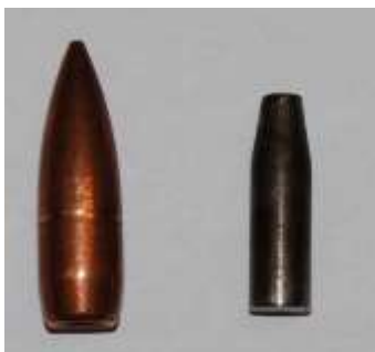
Figure 1.1.- Ammunition of calibre 7.62 x 39 mm M43 and its core.
