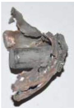
Figure 6.13.- Jacket surrounding the core after an impact.
