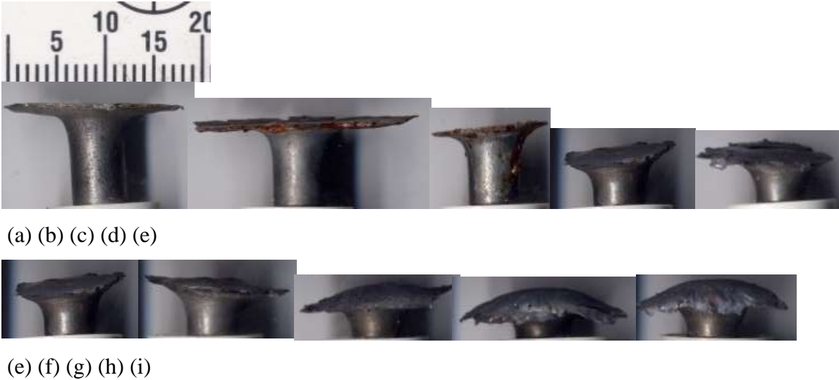
Figure 6.10.- Core after impacting rigid wall at (a) 486 m/s, (b) 550 m/s, (c) 572 m/s, (d) 797 m/s, (e) 838 m/s, (f) 842 m/s, (g) 920 m/s (h) 1016 m/s and (i) 1027 m/s.
