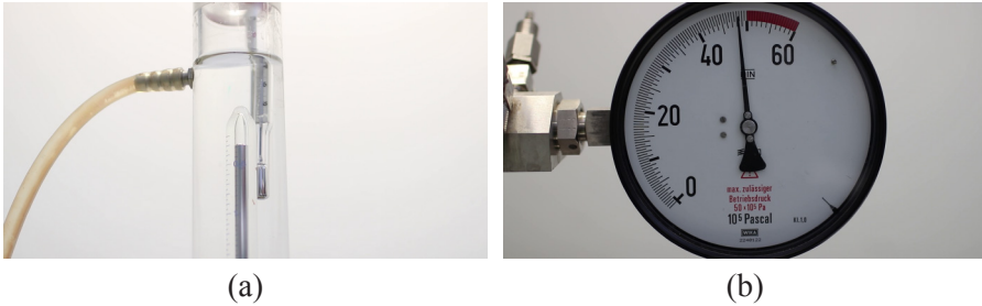
Figure 20. Attempt to reduce the volume of the liquid: (a) The volume almost does not vary; (b) Pressure increases sharply.
