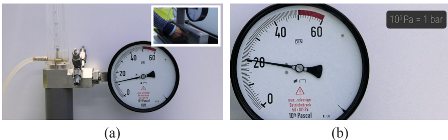
Figure 4. (a) Manometer and rotating wheel; (b) Maximum pressure 50 bar.
