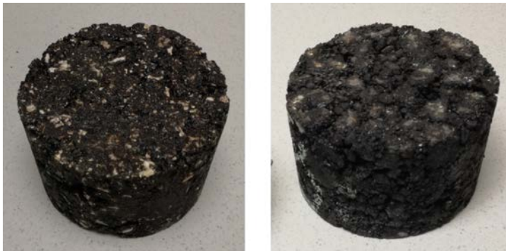
Fig. 2 – Specimens of CBB (left) and NBB (right) mixtures
