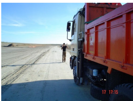
Figure 7. Wheel impression test: passing over the alignment pegs
