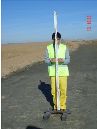
Figure 8. Wheel impression test: leveling over pikes
