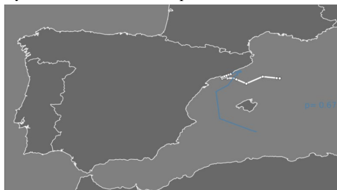
Figure 19: FP (white) and model prediction (blue) 4 hours before EOBT for flight #3229838 LIRF – LEBL.
