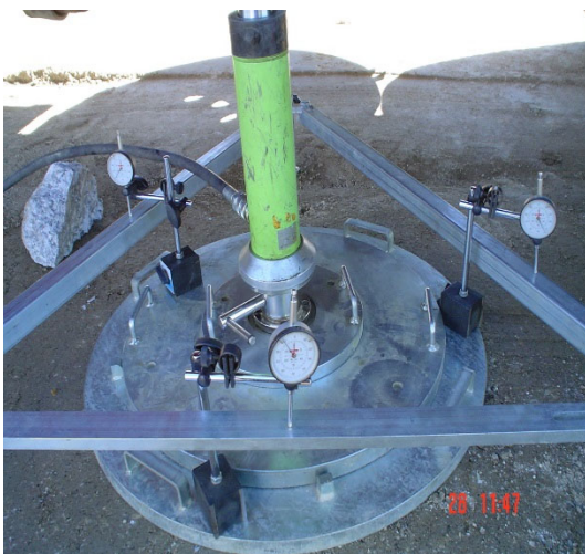
Figure 11. standard load plates (300, 600 and 762mm)
