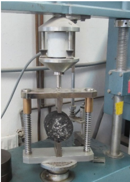
Fig. 2 - Indirect Tensile Strength Test
