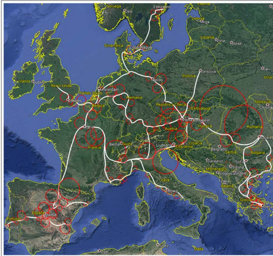
Figure 2: Curvature radii for a European Hyperloop Network
