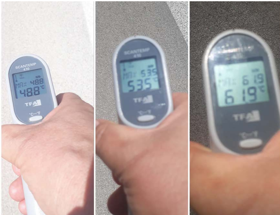
Fig. 18 – Thermometer. Surface temperatura difference dirty-clean 4,7 °C, conventional-cool pavement clean 13,1 °C (14/06/2020 - 15.30 a.m.).
