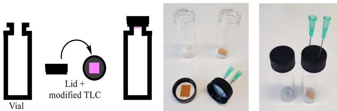
Fig. S4.32 Preparation and photos of the measurement vial using the immobilised probes.
