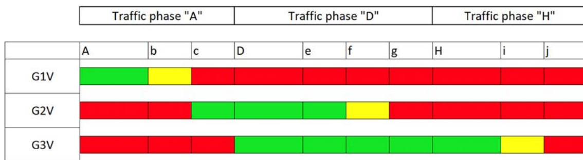
Fig. 2 – Example of phases for each signal group of an intersection
