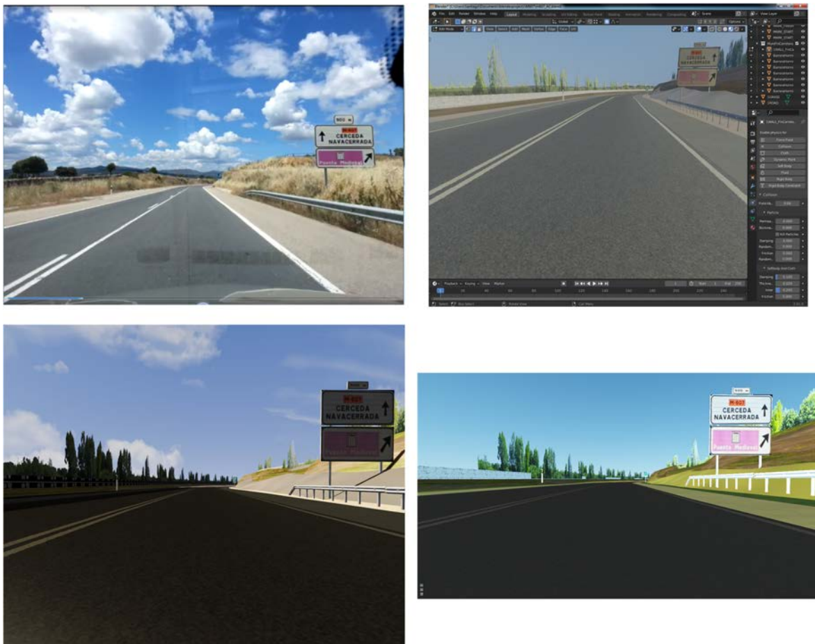
Figure 4 – Top left: a video recording of the actual road. Top right: image generated by Blender. Bottom left: image from Assetto Corsa. Bottom right: image from rFactor2
