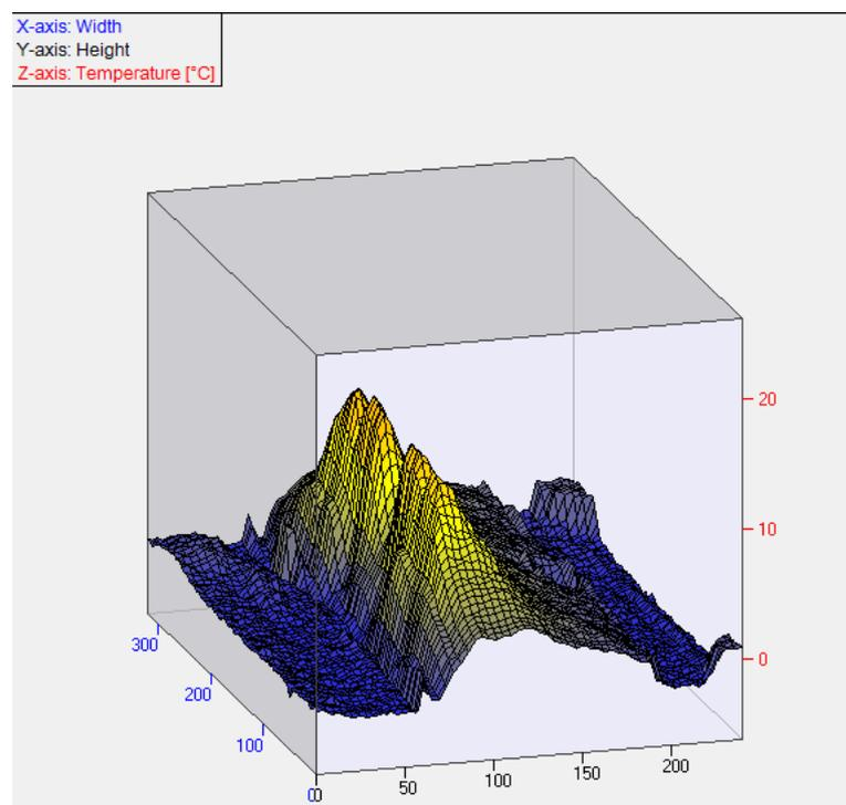
Figure 6: 3D graph of temperature on the windshield
