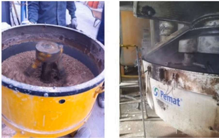
Fig. 3. Concrete mixers for mixes at laboratory scale (left) and at industrial scale (right).
