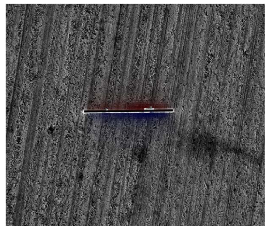
Figure 7: SEM image of the region in figure 6, after milling. The shading represents the intensity of the displacements detected by the FIB algorithm.
