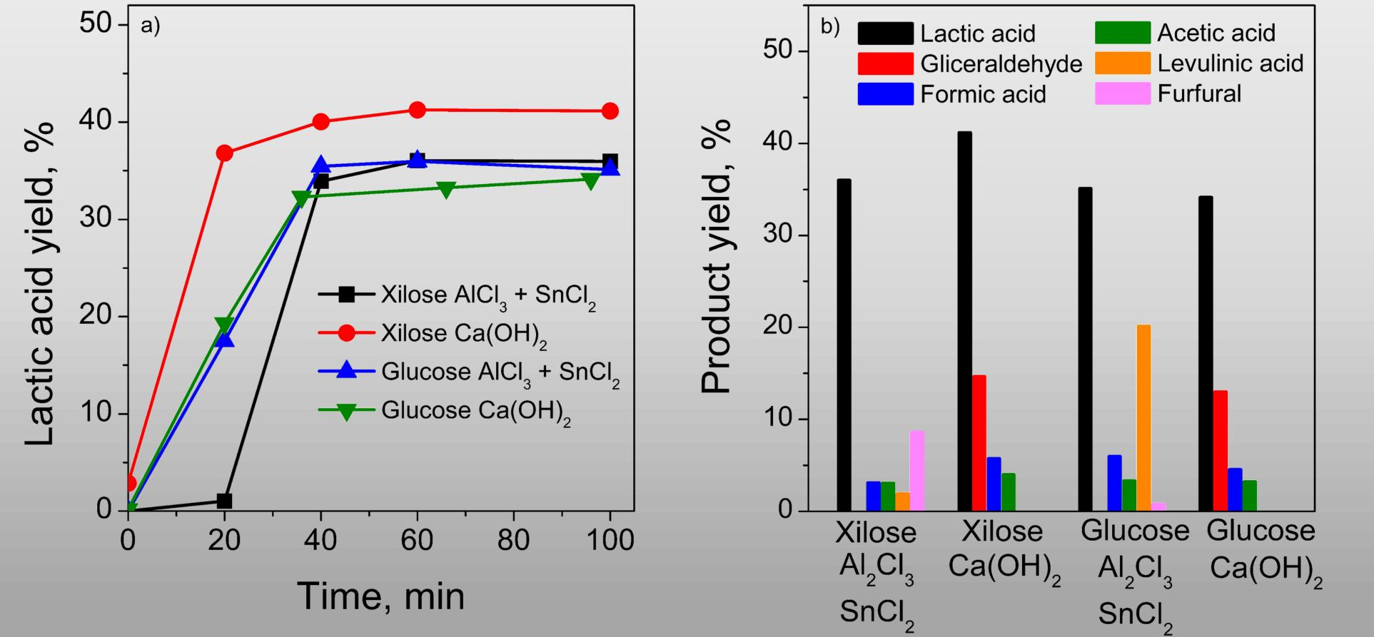
The presence of acid catalysts is more effective for glucose conversion; however, for xylose conversion base catalysts present a higher yield
