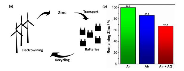
Figure 6 - 15. (a) Scheme of metallic zinc as energy carrier used in mechanicallyrechargeable Zn–Air batteries. (b) Results of experiments for determining the amount of zinc that remains when it is store in different media: Argon, Air and Air with 2,6-DHAQ.
