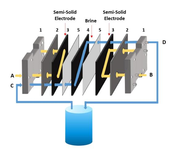
Figure 7 - 3. Flow diagram Membrane Free Ion Pumping Injectable Cell 1. 3D Printed ABS Endplate; 2. Graphite Current Collector; 3 and 4. Viton Gasket; 5. Microporous Separator C3501.
