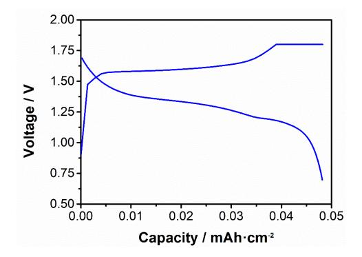
Figure 5 - 14. Voltage profiles for full cycles when a float charging protocol is applied (1.8 V for 15 min).
