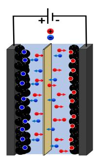
Figure 1 - 2. Scheme of the charge process of a supercapacitor. Movement of cations (red) and anions (blue).
