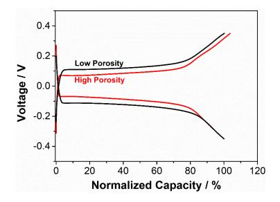
Figure 4 - 13. Normalized voltage profile of a  $FePO_4 - LiFePO_4$  injected battery with lower electrode porosity (70 vol%) cycled at 1 mA cm<sup>-2</sup> and higher electrode porosity (90 vol%) at 2 mA cm<sup>-2</sup>.
