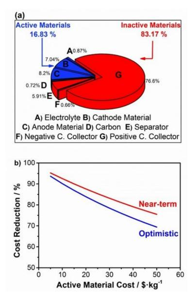
Figure 4 - 14. (a) Contributions of different elements to the cost of materials for the aqueous  $LiTi_2(PO_4)_3 - LiFePO_4$  battery. (b) Evolution of the contribution of inactive materials, which represents the reduction in battery costs, as a function of the active materials cost for an aqueous battery (neutral pH electrolyte). The values were calculated using prices of materials shown in Table 4-2.
