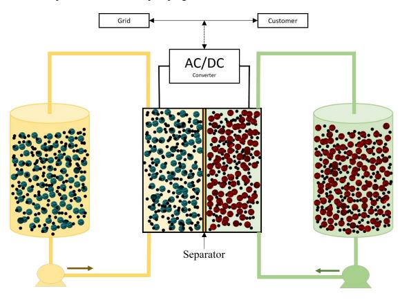
Figure 1 - 8. Scheme of a semi-solid redox flow battery.
