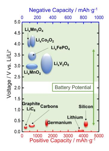
Figure 1 - 7. Representation of specific capacity and operating redox potential of various materials for Li-ion batteries, adapted with permission from [45].
