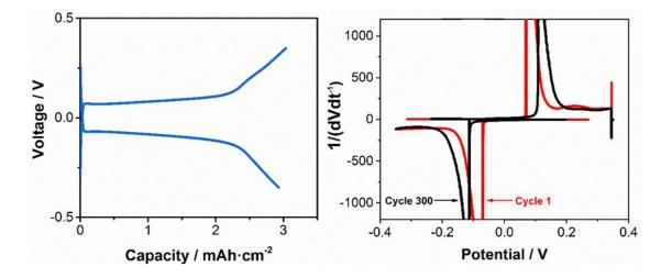
Figure 4 - 10. Voltage profile and differential voltage curves of the aqueous  $FePO_4 - LiFePO_4$ injectable battery for the 1<sup>st</sup> and 300<sup>th</sup> cycle at 2 mA cm<sup>-2</sup>. Electrode thickness: 2 mm and 1 mm for FePO<sub>4</sub> and LiFePO<sub>4</sub> semi-solid electrode, respectively.
