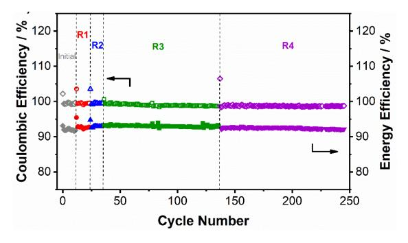
Figure 4 - 19. Energy and coulombic efficiency of Li - LiFePO<sub>4</sub> 0.3 mA cm<sup>-2</sup>.
