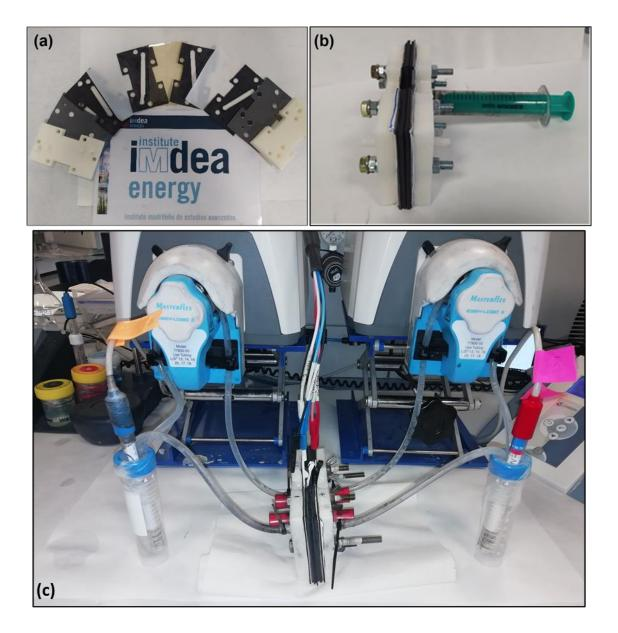
Figure 7 - 6. Pictures of (a) the different components of the Regenerative Electrochemical Ion Pumping Cell (3D Printed ABS Endplate, Graphite Current Collector, Viton Gasket, Microporous Separator C350, Anion Exchange Membrane (AEM), (b) regeneration process by dejection / injection of semi-solid electrode from / into the assembled REIP cell, (c) operating REIP system.
