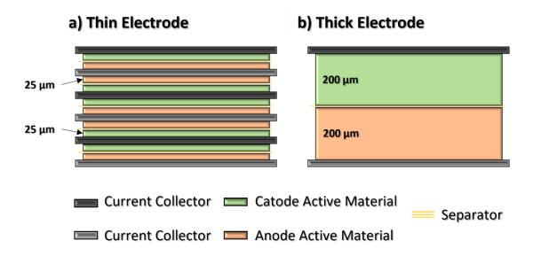
Figure 1 - 9. Different configurations of static battery (a) Conventional thin electrodes vs. (b) Thick electrodes. Adapted with permission from [115].
