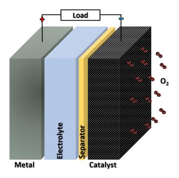
Figure 1 - 5. Illustration of the elements of a Metal - Air battery.
