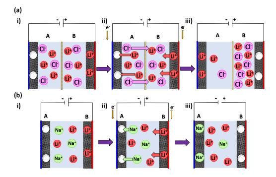
Figure 7 - 4. Illustration of two operating modes for the EIPC for the first half-cycle resulting in the concentration of Li-ions. (a). EIPC with ion-selective exchange membrane (b) Membrane free EIPC.
