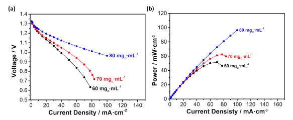
Figure 6 - 8. Performance of semi-solid electrodes with different formulation in terms of (a) Evolution of the operating voltage (b) Evolution of the specific power with the applied current density for a Zn content of 0.5 kg  $L^{-1}$ .
