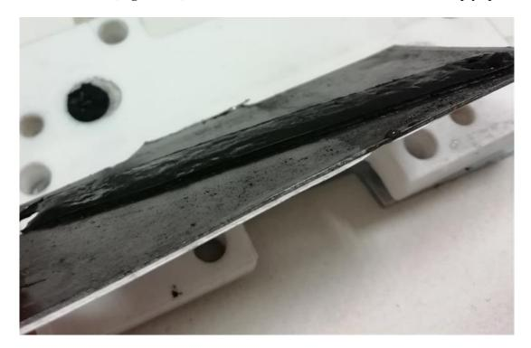
Figure 4 - 2. Photograph of the semi-solid electrode after dismantling the cell.
