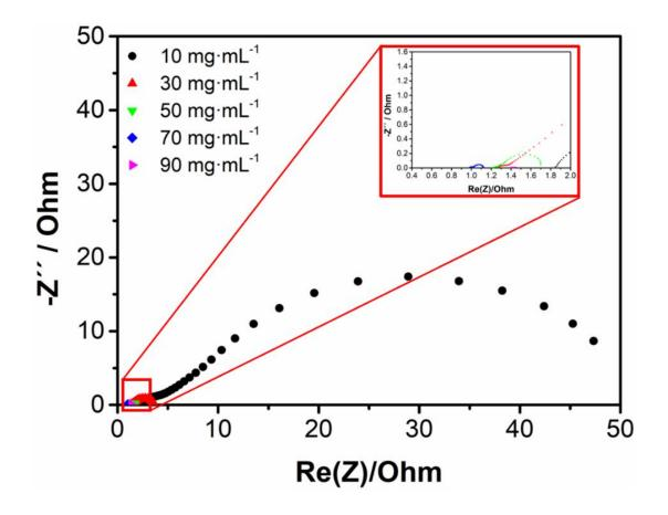
Figure 3 - 6. Nyquist plots of the EIS measurements for semi-solid electrodes containing 10, 30, 50, 70 and 90 mg<sub>carbon</sub> mL<sup>-1</sup>
