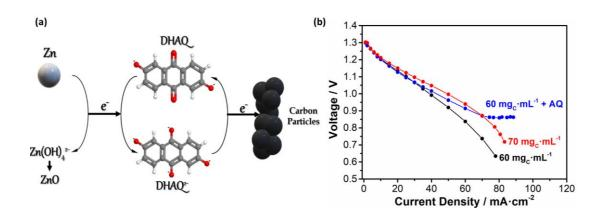
Figure 6 - 13. (a) Scheme of 2,6-dihydroxyanthraquinone acting as molecular wiring for mechanically rechargeable semi-solid Zinc-Air battery. (b) Comparison of the operating voltage when 2,6-dihydroxyanthraquinone is included into the formulation of the electrode.
