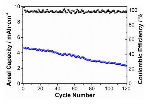
Figure 5 - 1 Cyclability test of an injectable  $Zn - MnO_2$  battery using semi-solid electrodes at 0.5 C.
