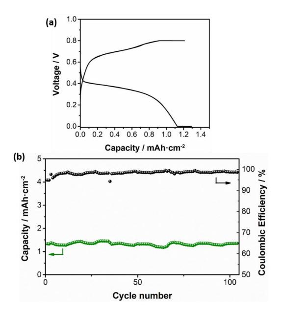
Figure 7 - 13. (a) Voltage profile and (b) cyclability test of the REIPC using an asymmetrical system (LFP-MO).
