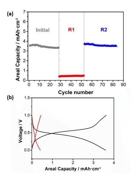
Figure 7 - 18. (a) Evolution of the areal capacity of the MFREIPC MO-NiHCF cell with the number of cycles. Regenerations were conducted in cycle 28 (carbon-based semi-solid electrode replaced NiHCF semi-solid electrode) and cycle 52 (fresh semi-solid electrodes). (b) Comparison between capacitive (Activated Carbon-Activated Carbon, red line) and Faradaic (MO-NiHCF, black line) MF-REIPC.
