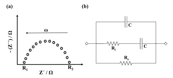
Figure 3 - 4. (a) Typical Nyquist plot for mixed ionic and electronic conductors, and (b) Equivalent electrical circuit.
