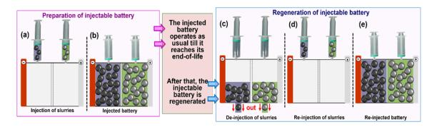
Figure 4 - 3. Illustration of the injectable battery concept. (a) The preassembled cell is fabricated, which is (b) filled with semi-solid electrode. After end-of-life (several years), the injectable battery regenerated by (c) removing the spent semi-solid electrodes, (d-e) having the cell ready for injecting fresh one.
