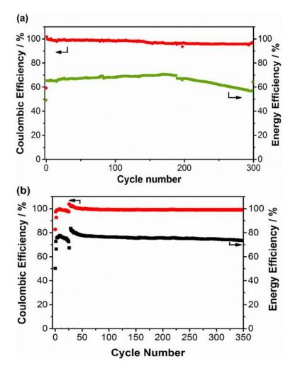
Figure 4 - 9. Energy and coulombic efficiency of aqueous (a)  $LiTi_2(PO_4)_3 - LiFePO_4$  and (b) super-concentrated Zn - LiFePO<sub>4</sub> injectable battery operated at 1 mA cm<sup>-2</sup> and 2 mA cm<sup>-2</sup>, respectively.
