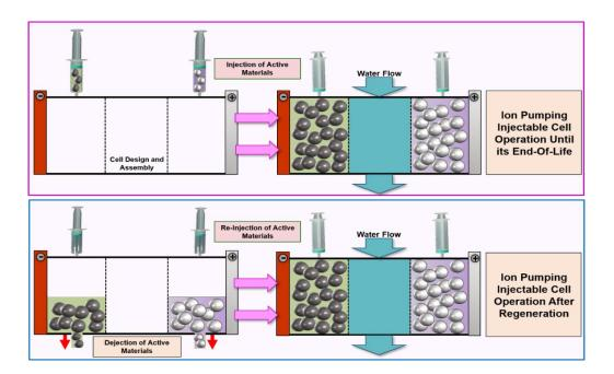
Figure 7 - 5. Process of substitution (injection and dejection) of the semi-solid electrodes into a pre-assembled cell for their use in ion pumping applications.
