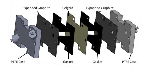
Figure 4 - 6. Schematic representation of the cell design of the aqueous super-concentrated Zn - LiFePO<sub>4</sub>, FePO<sub>4</sub> - LiFePO<sub>4</sub> and LiTi<sub>2</sub>(PO<sub>4</sub>)<sub>3</sub> - LiFePO<sub>4</sub> injectable battery.
