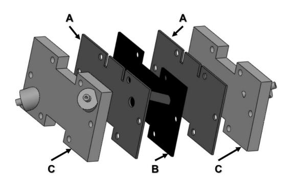
Figure 3 - 3. Design scheme of the separator-free symmetrical cell containing (A) Expanded graphite, (B) Gasket and (C) ABS 3D printed case.
