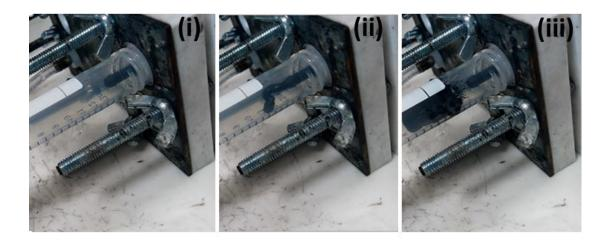
Figure 6 - 3. Removal of the semi-solid electrode from a filled battery cell. (i) Initially, the cell is filled with a semi-solid electrode. (ii) Air pressure is applied inside the cell through the one of the inlets, and the semi-solid electrode starts to come out of the cell. (iii) Finally, all the spent semi-solid electrode is removed from the cell, which is then empty and ready for being used again.
