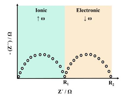
Figure 3 - 5. Nyquist plot for relevant mixed ionic and electronic transport.
