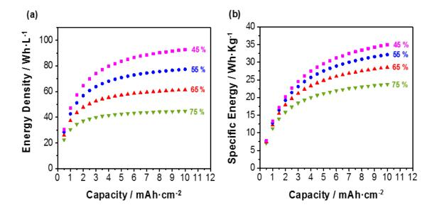
Figure 4 - 16. Evolution of (a) energy density and (b) specific energy as a function of the areal capacity and electrode porosity for the aqueous  $LiTi_2(PO_4)_3 - LiFePO_4$ .
