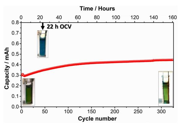
Figure 5 - 12 Evolution of the charge capacity when a float charging protocol is applied (1.8 V for 15 min). Inset: color of the electrolyte at the beginning, after 22 h at open circuit voltage (spontaneous drift towards alkaline values) and after 300 cycles implementing the float charging protocol. Total duration of the experiment was >160 h.
