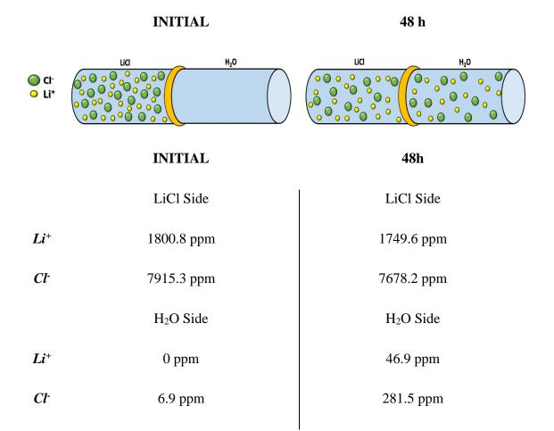
Figure 7 - 16. Experiment showing the permeability of the anion exchange membrane to the lithium ions.
