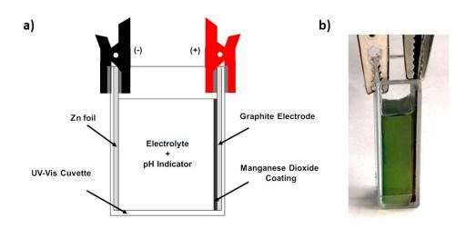
Figure 5 - 6 (a) Scheme of the Zn-MnO<sub>2</sub> cell assembled in a UV-Vis Cuvette. (b) Picture of the cell filled with electrolyte containing pH indicator. Green color indicates that the pH value is between 3 and 5.
