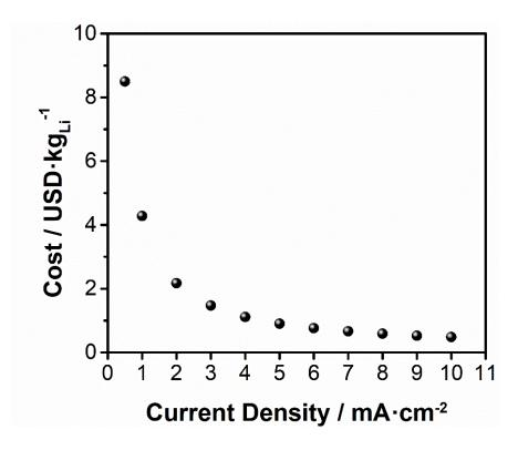
Figure 7 - 12. Operational costs of the system per kg of lithium recovered as a function of the current density.
