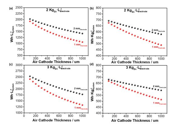
Figure 6 - 14. Theoretical estimation of energy density for Zn-Air batteries using semi-solid electrodes. Comparison between two different Zinc content in the electrode: (a) and (b) for  $2 \text{ kg}_{zn} \text{ L}^{-1}$ , and (c) and (d) for  $3 \text{ kg}_{zn} \text{ L}^{-1}$ . Thickness of Celgard separator and stainless-steel current collector are  $25\mu m$  and  $12\mu m$ , respectively.
