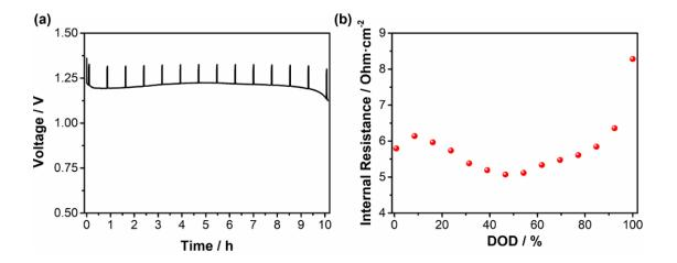
Figure 6 - 9. Voltage profile of a galvanostatic intermittent titration technique measurement at 20 mA cm<sup>-2</sup> for a semi-solid electrode containing 1 Kg<sub>Zn</sub>  $L^{-1}$  and 70 g<sub>C</sub>  $L^{-1}$ , and (b) the resulting evolution of the internal resistance with the depth of discharge.
