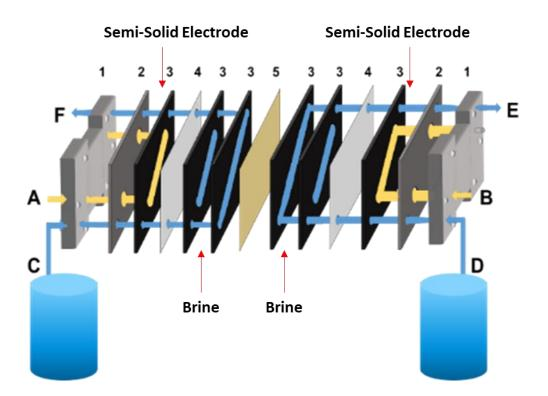
Figure 7 - 2. Flow diagram of Ion Pumping Injectable Cell 1. 3D Printed ABS Endplate; 2. Graphite Current Collector; 3. Viton Gasket; 4. Microporous Separator C3501; 5. Anion Exchange Membrane (AEM).
