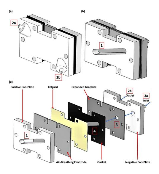
Figure 6 - 1. Design of the semi-solid Zn-air device fabricated using 3-D Fused Deposition Modelling Printing. (a) Packed cell (negative end-plate view). (b) Packed cell (positive endplate view). (c) Internal part of the cell.
