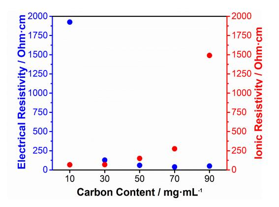
Figure 3 - 7. Electrical and ionic conductivities for semi-solid electrodes containing 10, 30, 50, 70 and 90 mg<sub>carbon</sub> mL<sup>-1</sup>.
