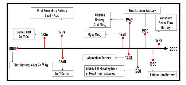
Figure 1 - 4. History of batteries. Timeline illustrating milestones achieved in the field of batteries in the last 200 years.
