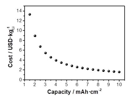
Figure 7 - 11. Installation cost per Kg of Li as a function of the areal capacity.
