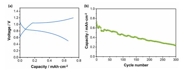
Figure 4 - 8. (a) Voltage profile and (b) evolution of the areal capacity with cycles for the  $LiTi_2(PO_4)_3 - LiFePO_4$  injectable battery.
