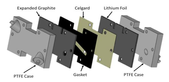
Figure 4 - 17. Schematic representation of the cell design of the non-aqueous Li – LiFePO<sub>4</sub> injectable battery.
