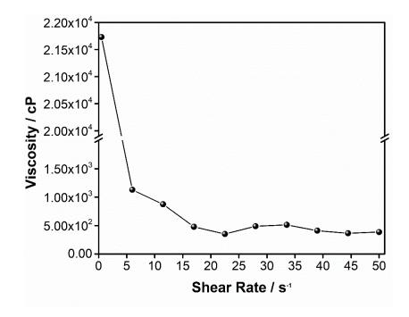
Figure 3 - 1. Rheological behavior of a semi-solid electrode containing LFP, carbon additive, and electrolyte.
