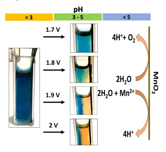
Figure 5 - 9. Pictures of the cuvette cell after open circuit voltage (left) and when a constant voltage of 1.7 V, 1.8 V, 1.9 V and 2.0 V was applied to the cell. Zn foil and  $MnO_2$  electrode are located at the left and right side of the cuvette. Right: scheme of the electrochemical reaction taking place at the positive electrode.
