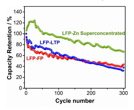
Figure 4 - 11. Comparison of capacity retentions for the  $LiTi_2(PO_4)_3 - LiFePO_4$ , the superconcentrated  $Zn - LiFePO_4$  and the  $FePO_4 - LiFePO_4$  injectable batteries. An average capacity decay of 0.15, 0.13 and 0.08 % cycle<sup>-1</sup>, respectively, was calculated for the last 200 cycles.
