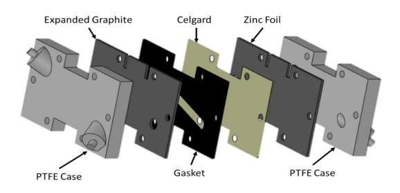
Figure 4 - 4. Schematic representation of the cell design of the  $Zn - LiFePO_4$  injectable battery.
