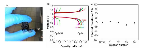
Figure 4 - 5. (a) Photograph of a semi-solid electrode. (b) Voltage profile of an injected  $Zn - LiFePO_4$  battery in the 1<sup>st</sup> and 50<sup>th</sup> cycle for the initial battery and after 4 subsequent regenerations (R1, R2, R3 and R4) at 1C (2.5 mA cm<sup>-2</sup>). (c) Variation of the internal resistance of the injectable battery with respect to initial value when semi-solid electrodes are substituted.
