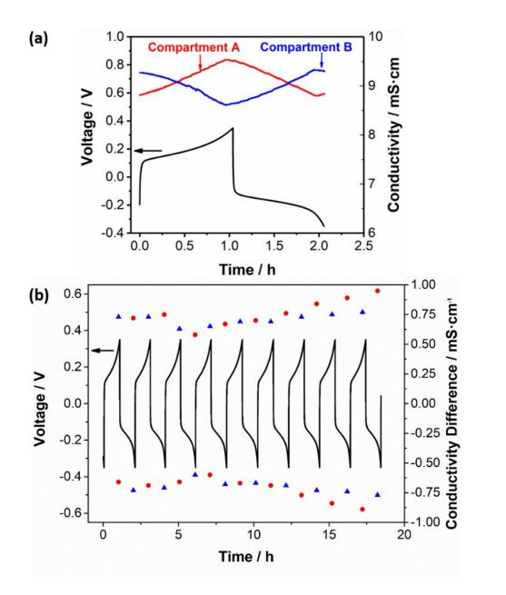
Figure 7 - 15. Evolution of cell voltage and ionic conductivity of the symmetrical REIPC during (a) one full cycle and (b) ca. 20 h. Blue triangles and red circles represent the conductivity difference values in each one of the compartments at the end of each one of the charging/discharging cycles.
