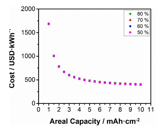
Figure 4 - 15. Evolution of cost of materials as a function of the areal capacity and electrode porosity for an aqueous  $LiTi_2(PO_4)_3 - LiFePO_4$  battery.
