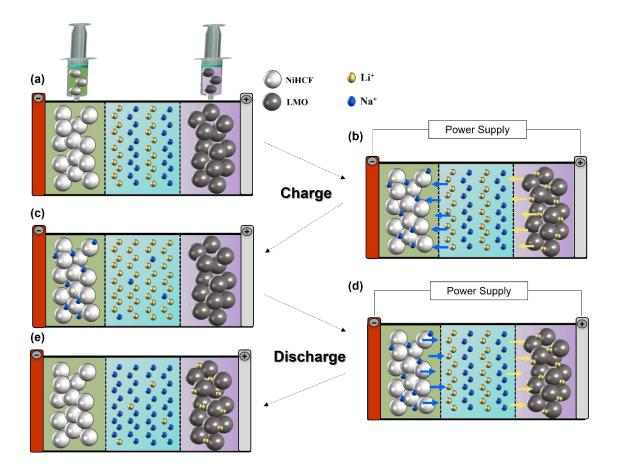
Figure 7 - 17. Graphical explanation for the movement of the ions (Na+ and Li+) in the MF-REIPC system with LMO-NiHCF electrodes. (a-c) Charging process, concentration of lithium ions in the solution. (c-e) Discharging process, concentration of sodium ions in the solution.
