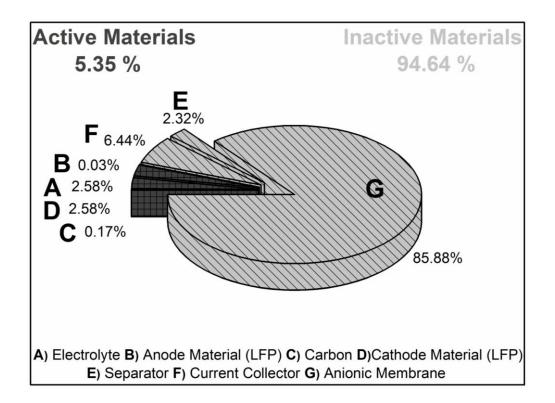
Figure 7 - 9. Contribution of different elements to cost of a REIPC: inactive and active materials.
