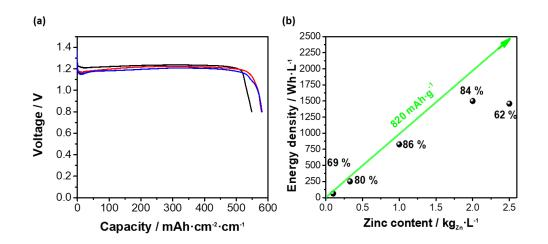
Figure 6 - 5. (a) Voltage profiles of three subsequent injections. (b) Energy density evolution for semi-solid electrodes with different zinc content (0.1 kg<sub>Zn</sub>  $L^{-1}$ , 0.33 kg<sub>Zn</sub>  $L^{-1}$ , 1 kg<sub>Zn</sub>  $L^{-1}$ , 2 kg<sub>Zn</sub>  $L^{-1}$  and 2.5 kg<sub>Zn</sub>  $L^{-1}$ ).
