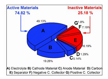
Figure 4 - 20. Contributions of different elements to the cost of materials for a non-aqueous Li - LiFePO<sub>4</sub> battery.
