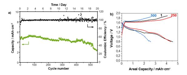
Figure 5 - 4 (a) Cyclability test of the hybrid system: injected  $MnO_2$  - Zn-foil with electrolyte flow. (b) Voltage profiles of  $1^{st}$ , 250<sup>th</sup> and 500<sup>th</sup> cycles.
