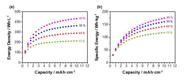
Figure 4 - 21. Evolution of (a) Energy density and (b) Specific energy as a function of the areal capacity and electrode porosity for a non-aqueous  $Li - LiFePO_4$  battery.
