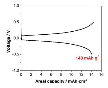
Figure 4 - 12. Voltage profile of a  $FePO_4 - LiFePO_4$  injected battery with an electrode porosity of 70 vol% cycled at C/14 (1 mA cm<sup>-2</sup>) reaching a utilization rate of  $LiFePO_4$  of 140 mAh g<sup>-1</sup> for the limiting side (the 1 mm-thick electrode vs the 2 mm-thick electrode).
