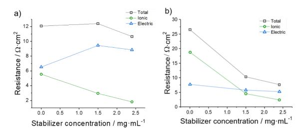
Figure 3 - 9. (a) Ionic, electrical, and total conductivity of a semi-solid electrode for 42 mg mL<sup>-1</sup> carbon additive. (b) Ionic, electrical, and total conductivity of a semi-solid electrode for 53 mg mL<sup>-1</sup> carbon additive.
