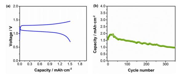
Figure 4 - 7. (a) Voltage profile and (b) evolution of the areal capacity with cycles for the superconcentration  $Zn - LiFePO_4$  injectable battery in 21 m LiTFSI and 1 m ZnTFSI.
