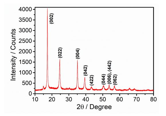
*Figure 7 - 1. XRD pattern of Potassium Nickel Hexacyanoferrate (KNi[Fe(CN)<sub>6</sub>]) matching the diffraction previously reported for this materials.* <sup>26</sup>
