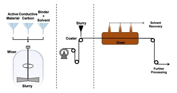
Figure 1 - 10. Illustration of the manufacturing process of conventional electrodes. Adapted from [119].
