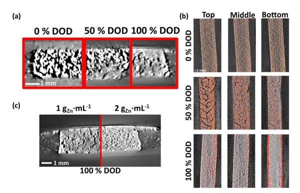
Figure 6 - 7. X-ray computed tomography (a) Cross section of semi-solid electrodes at different Depth-Of-Discharge (0 %, 50 % and 100 %). (b) Top-view of electrodes at different semi-solid heights (top, bottom, and middle) with different DOD. (c) Cross section of two electrodes with different Zn content (1 kg<sub>Zn</sub>  $L^{-1}$  and 2 kg<sub>Zn</sub>  $L^{-1}$ ) at 100 % DOD.
