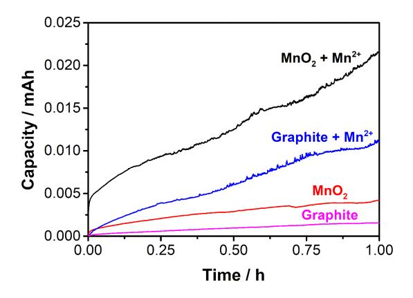
Figure 5 - 10. Accumulated charge consumed with time when a constant voltage of 1.8 V is applied during one hour in four systems: Graphite as positive electrode with (blue) and without (pink)  $Mn^{2+}$  additive in the electrolyte, and  $MnO_2$  electrode as positive side with (black) and without (red)  $Mn^{2+}$  additive in the electrolyte.
