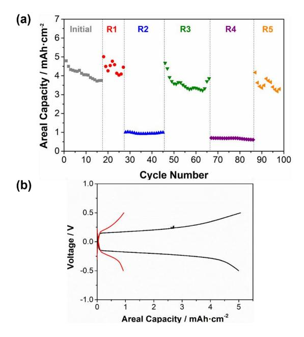
Figure 7 - 7. Performance of the REIPC LFP-FP cell. (a) after several injections and reinjections with activated carbon and LFP. (b) Comparison between capacitive (Activated Carbon-Activated Carbon, red line) and Faradaic (LFP-FP, black line) REIPC Cells.
