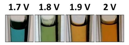
Figure 5 - 11. Pictures of the electrolyte after a constant voltage of 1.7 V, 1.8 V 1.9 V and 2.0 V was applied for 2 h.
