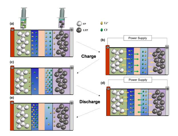
Figure 7 - 14. Graphical explanation for the movement of the ions (Cl<sup>-</sup> and Li<sup>+</sup>) in the REIPC system with symmetrical LFP configuration. (a-c) Charging process, concentration of the solution in the positive side and dilution in the negative. (c-e) Discharging process, dilution of the solution in the negative side and concentration in the positive.
