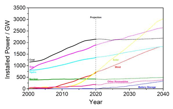
Figure 1 - 1. Installed power capacity. Adapted with permission from [1].
