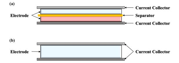
Figure 3 - 2. Cell design for (a) Conventional battery and (b) Separator-free configuration for determination of electrical properties of semi-solid electrodes.
