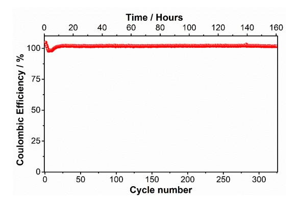
Figure 5 - 13. Coulombic efficiency for a Zn-MnO2 cell when a float charging protocol is applied (1.8 V for 15 min.
