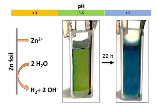
Figure 5 - 7 Spontaneous evolution of the electrolyte pH without the application of an external bias.
