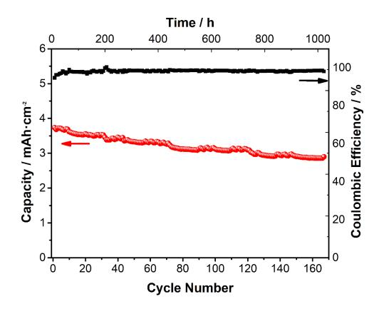
Figure 7 - 19. Cycling experiment probing the stability of the MF-REIPC system after being regenerated.
