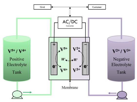
Figure 1 - 6. Scheme of an all-Vanadium redox flow battery.
