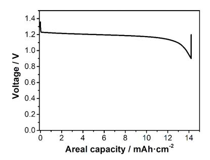
Figure 6 - 11. Voltage profile of a Zn-Air battery using stainless steel as current collector.
