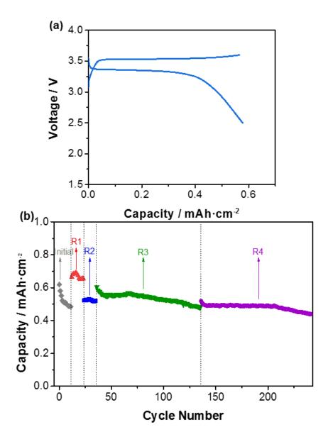
Figure 4 - 18. (a) Voltage profile and (b) evolution of the area capacity with cycles for 4 subsequent regenerations for the non-aqueous  $Li - LiFePO_4$  injectable battery electrode.
