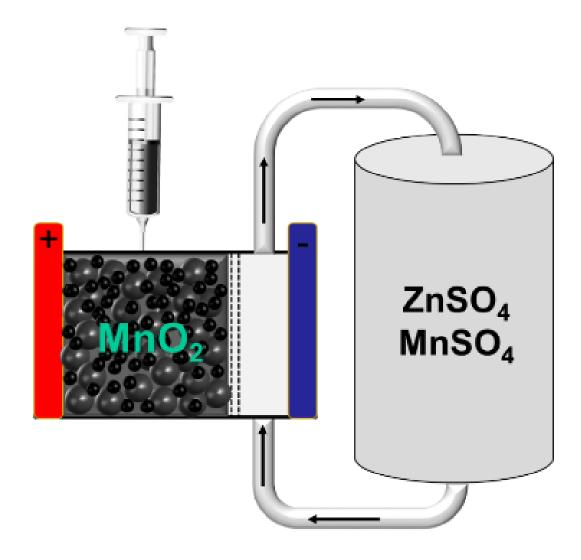
Figure 5 - 2 Scheme of the battery cell design for the hybrid-flow injectable  $Zn - MnO_2$  battery.
