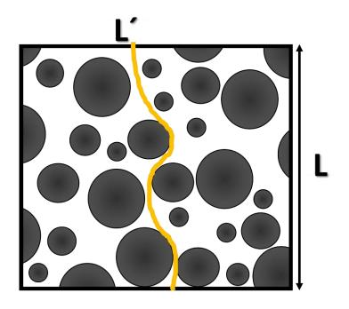
Figure 1 - 11. Drawing representing the tortuosity of a porous media.
