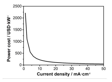
Figure 6 - 12 Evolution of power cost with current density
