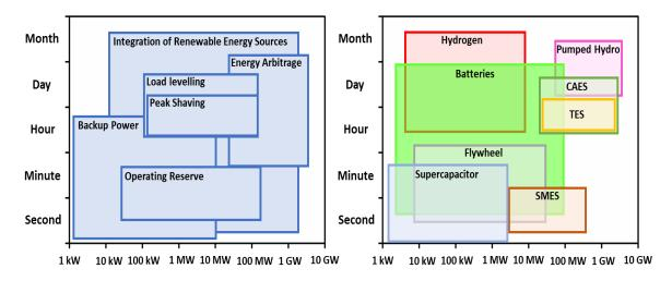
Figure 1 - 3. Time of energy release and power rate for (a) Energy storage applications and (b) Energy storage systems. Adapted with permission from [25].
