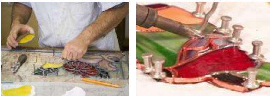
Figure 1.4: Assembly of glass pieces (left) and soldering lead comes (right). (©Traditional Craft).
