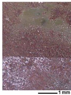
Figure 5.32: Green glass from Cuenca cathedral. A close up optical image of section f in figure 5.31 after laser cleaning at a laser energy value of 1.34 \mu\text{J}/\text{pulse} with a single irradiation series. The top part is the laser cleaned area also showing the uneven distribution of the red-brown grisaille.
