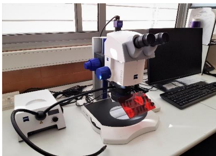
Figure 2.8: ZEISS SteREO Discovery.V8 optical microscope used in the surface morphological observation of the glasses. INMA-CSIC University of Zaragoza, Spain.
