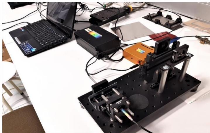
Figure 2.10: Spectrometer setup used to measure the transmittance of the glasses. In the foreground is a glass piece in the sample holder. INMA-CSIC University of Zaragoza, Spain.
