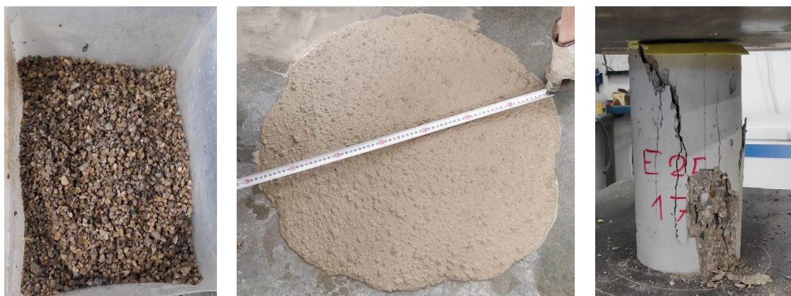
Figure 2. Highlights of the experimental plan: coarse RCA pre-soaked (left), slump-flow test of mix SA50 (middle), and specimen tested for compressive strength (right).
