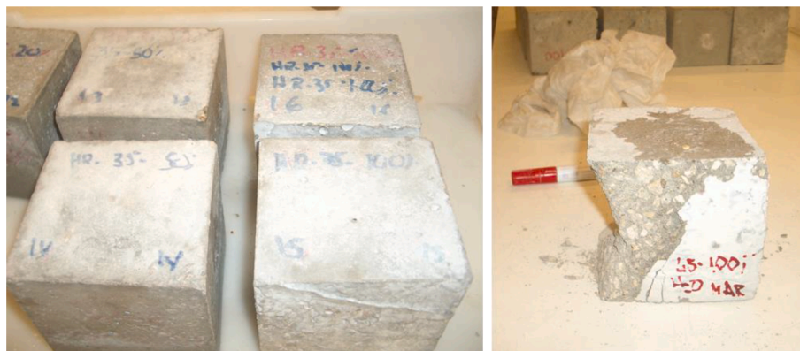
Fig. 13. Appearance of specimens after completion of the marine-water moist/dry test.
