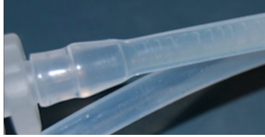
Figure 2: Experimental image showing a biofilm helix wrapped around the tube wall past the junction. No biofilm is formed in the unperturbed branch. Bacteria were injected upstream the junction.
