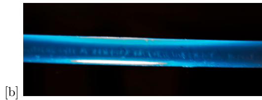
Figure 3: Experimental image showing the onset of a helical instability along a biofilm thread in a 2mm diameter tube.
