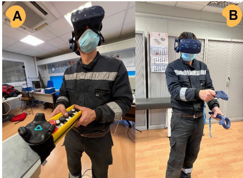
Fig. 3. Crane operator testing the different methods of interaction. A: real bridge crane controller. B: general virtual reality controllers.
