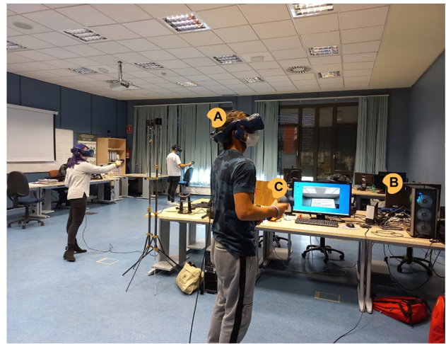
Fig. 4 User setup during the tutorial A HTC Vive Pro Eye HMDs and C its hand-controllers connected to B the workstation equipped with Intel Core i7-10710U, 32 GB RAM, with NVIDIA GTX 2080 graphic cards
