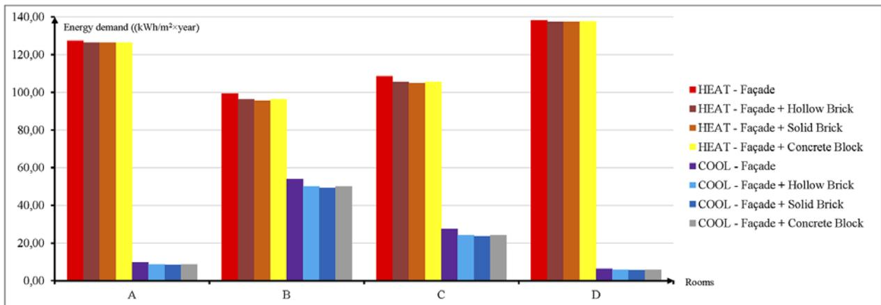
Fig.7. Results of the energy simulations related with the façades thermal inertia.
