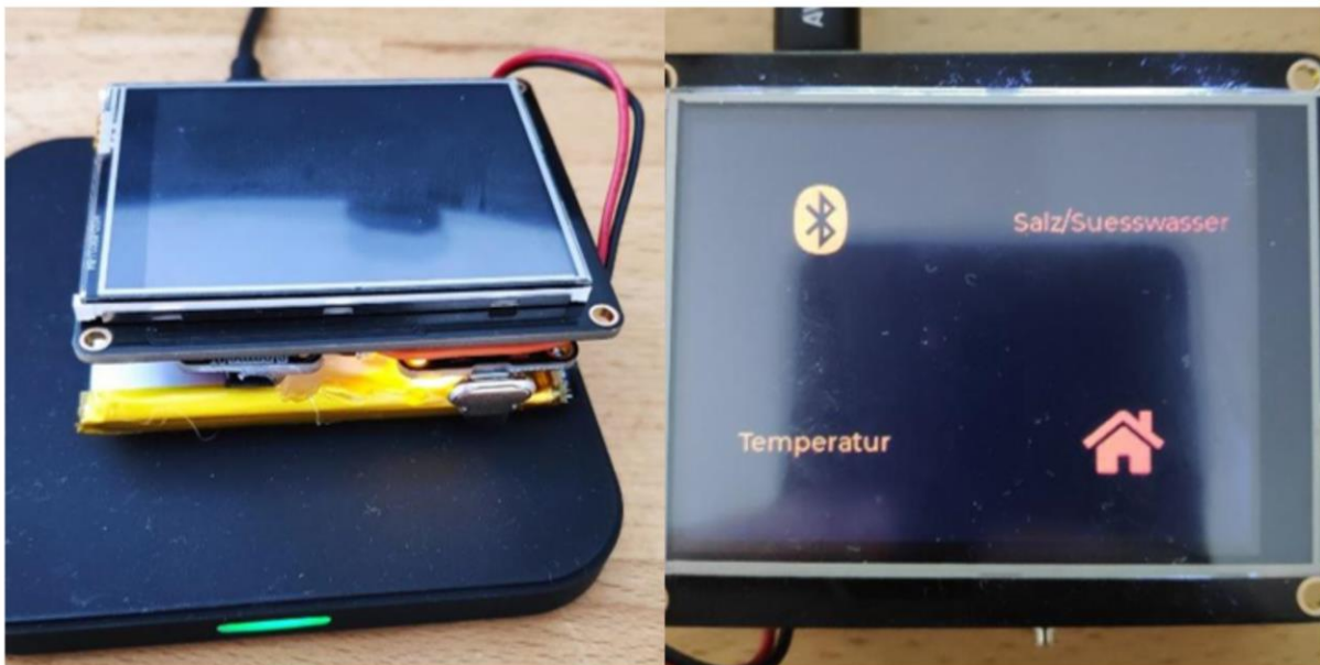
FIGURE 22. LEFT: THE DIVE COMPUTER CHARGING WIRELESS WITHOUT HOUSING. RIGHT: DIVE COMPUTERS SETTINGS SCREEN
