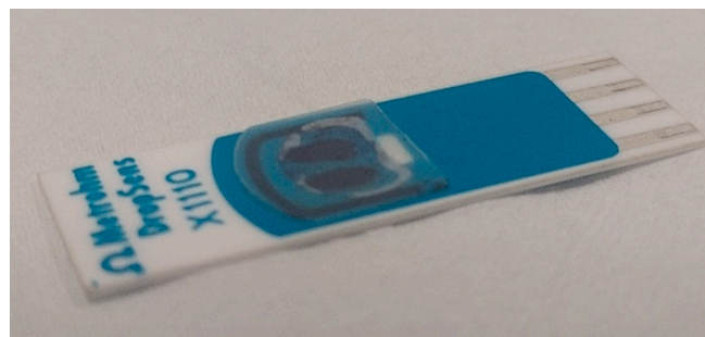
Fig. 1. AC_{60} and CoPh modified dual SPCEs, coated with a commercial polyamide membrane, for the simultaneous detection of 4-ethylphenol and ethanethiol.
