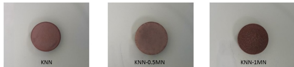
Figure 7. Pictures of KNN-xMN sintered pellets.
