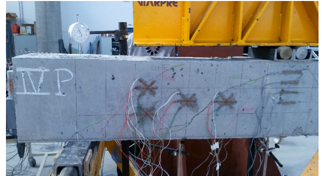
Fig. 7. Left shear span of IVP beam.
