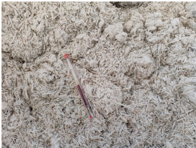
Fig. 3. Raw-crushed wind-turbine blade.
