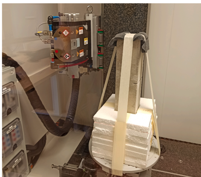
Fig. 2. Preparation of ‘S’ size specimens for CT scanning.
