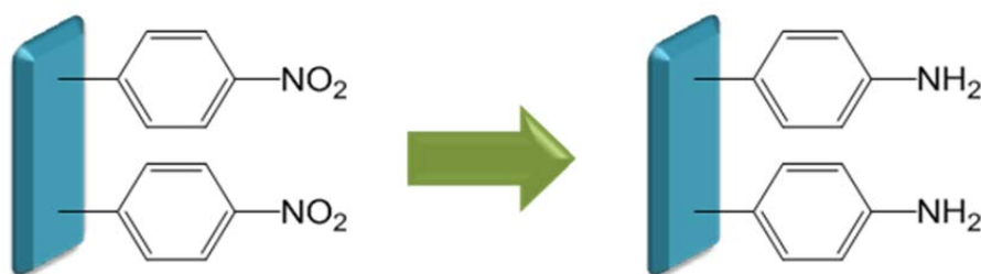
Figure 5.8.- Reduction of the nitro groups on the functionalised working electrode.
