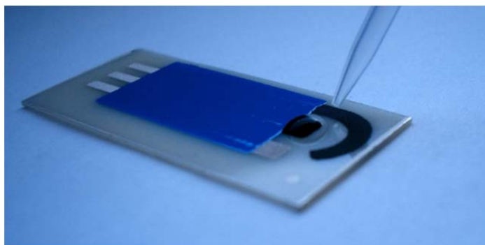
Figure 5.12.- Deposition of the enzyme, EDC and NHS solutions on the functionalised surface of the working electrode.
