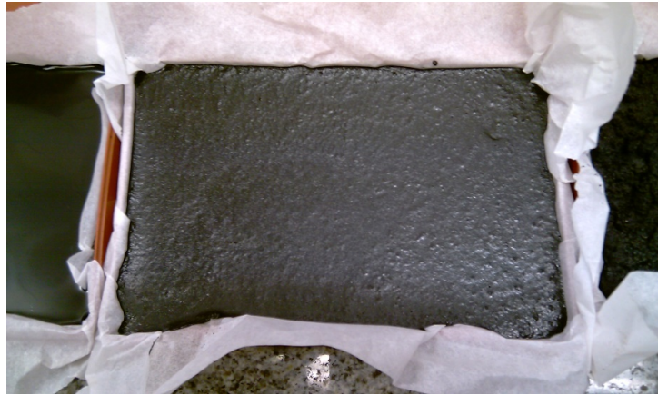
Figure 1.6. Modified bitumen with PU foam wastes
