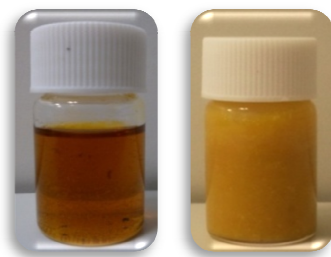
Figure 2.2. Example of the oils obtained at 25 MPa and 40 °C (R2, left) and 55 MPa and 70 °C (R7, right)
