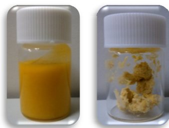
Figure 2.6. Examples of extracts obtained in the two-stage SFE: first stage (left) and second stage (right)
