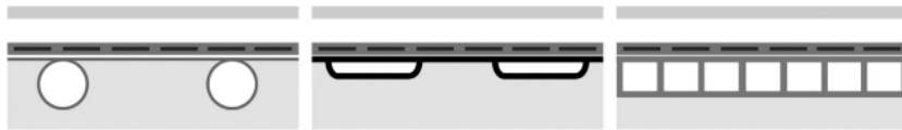
Figure S.9: Different tube sections for the thermal collector of a PV/T panel [35]
