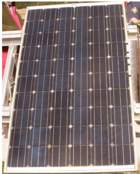
Figure S.24: Second prototype PV/T panel installed.
