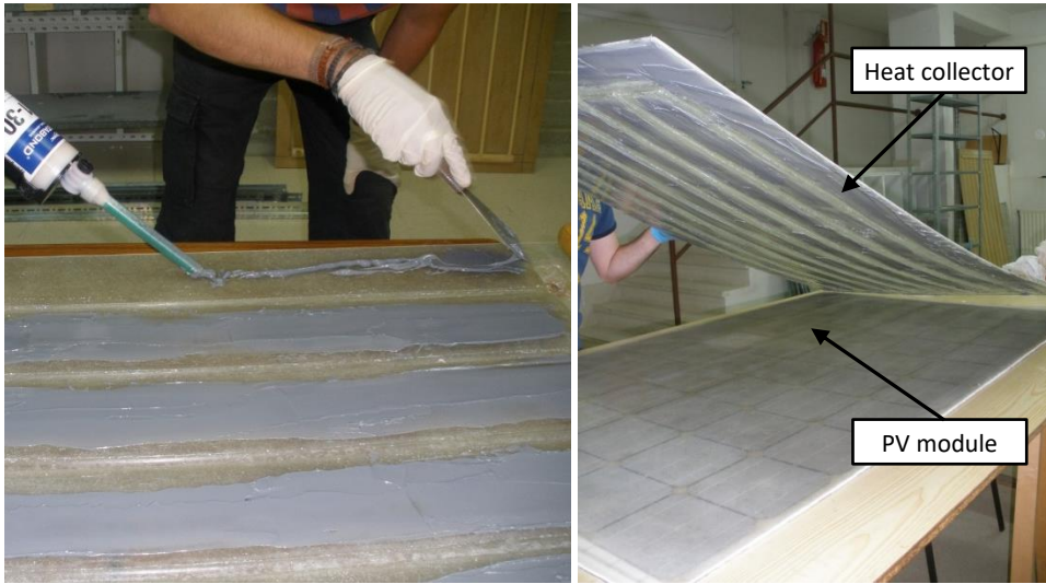
Figure S.23: Application of Crestabond M1-30 adhesive on the thermal collector (left) and assembly of the PV/T panel (right)
