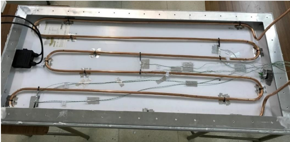
Figure S.25: PV/T + PCM prototype with thermal collector and thermocouples placed.
