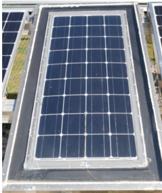
Figure S.29: PV/T panel prototype with heat storage by PCM and heat pipe to improve the PCM melting process
