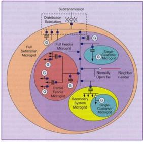
Figure 5. Future Power System Structure Source: IEEE Power & Energy. Vol.14, Number 5, September/October 2016
