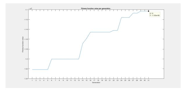
Figure 26. Evolution of the Fitness Function Value for the Power Distribution Grid Optimization Problem
