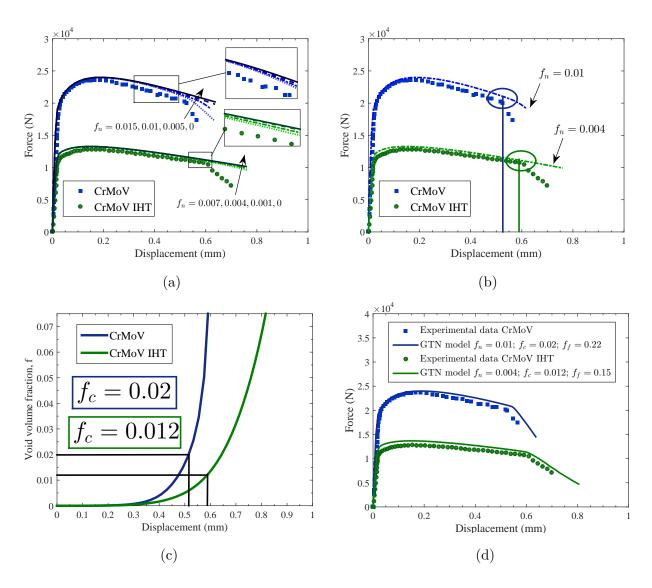
Figure 17: Outline of the top-down approach: (a) Experimental data and numerical predictions for different values of  $f_n$ , (b) identification of the sudden load drop associated with void coalescence, (c) void volume fraction in the center of the specimen versus displacement for the chosen value of  $f_n$ , (d) numerical damage simulation.
