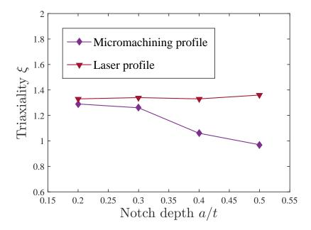
Figure 11: Triaxiality levels in the direction of maximum  $\xi$  at  $r\sigma_y/J=1$  for a longitudinal notch (L) resembling laser and micromachining fabrication techniques, different notch depths and t=0.5 mm.
