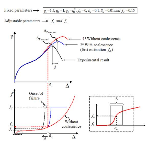
Figure 14: Outline of the proposed methodology to identify the GTN parameters from a notched SPT specimen.
