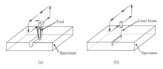
Figure 10: Schematic view of (a) high-precision micromachining and (b) laser-induced micromachining notch fabrication approaches.
