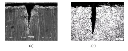
Figure 13: Cross section of the notch obtained from (a) laser-induced micromachining and (b) femtolaser-induced micromachining.
