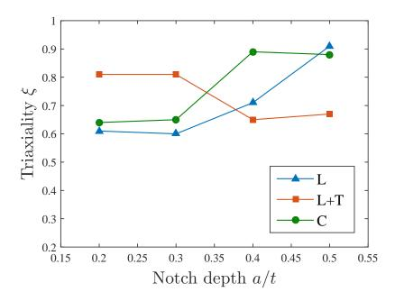
Figure 6: Triaxiality levels in the direction of fracture at  $r\sigma_y/J=1$  for several notch types, different notch depths and t=0.5 mm.
