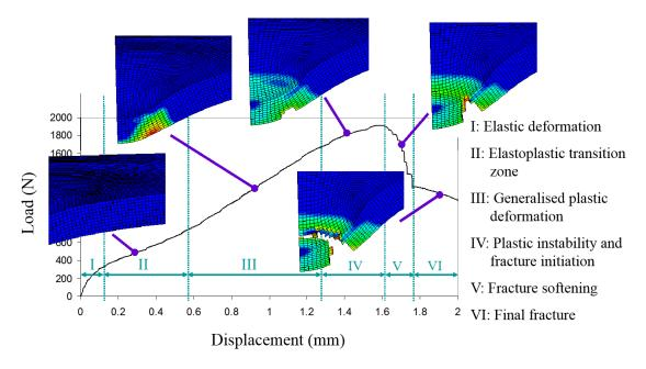
Figure 3: Regions of the load - punch displacement curve in a Small Punch Test
