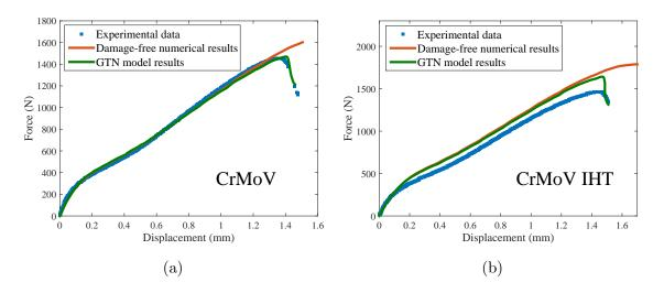
Figure 18: SPT experimental and numerical (with and without damage) load-displacement curves for (a) CrMoV and (b) CrMoV IHT
