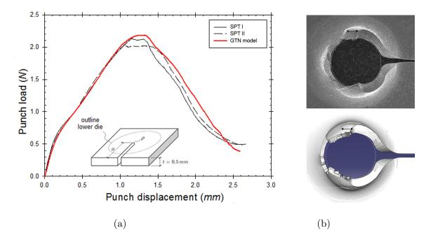
Figure 15: Numerical and experimental correlation for SPT expecimens with an edge notch: (a) Load-displacement curve and (b) crack growth predictions. The crack length equals 5 mm.
