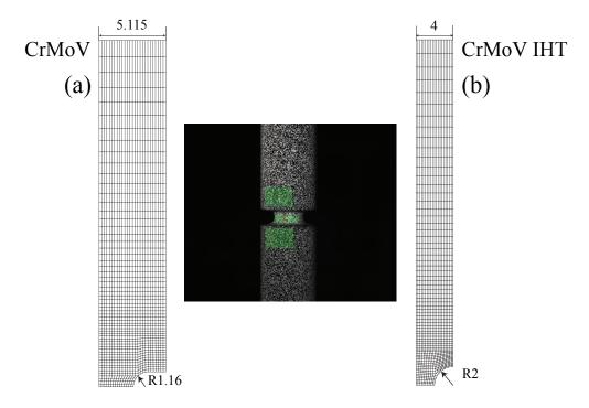
Figure 16: Mesh and geometry of the notched uniaxial tensile specimens employed for (a) CrMoV and (b) CrMoV IHT; a representative image of the DIC characterization is also shown. All dimensions are given in mm.
