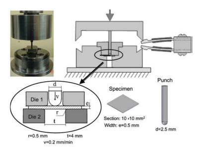
Figure 2: Device and schematic description of the Small Punch Test
