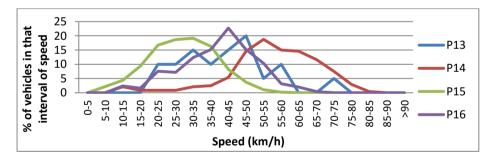
Fig. 12. Speed profile at zones 3 and 4.
