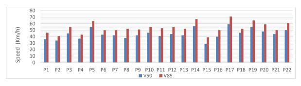
Fig. 9. V50 and V85 speed measured at the 22 street sections.
