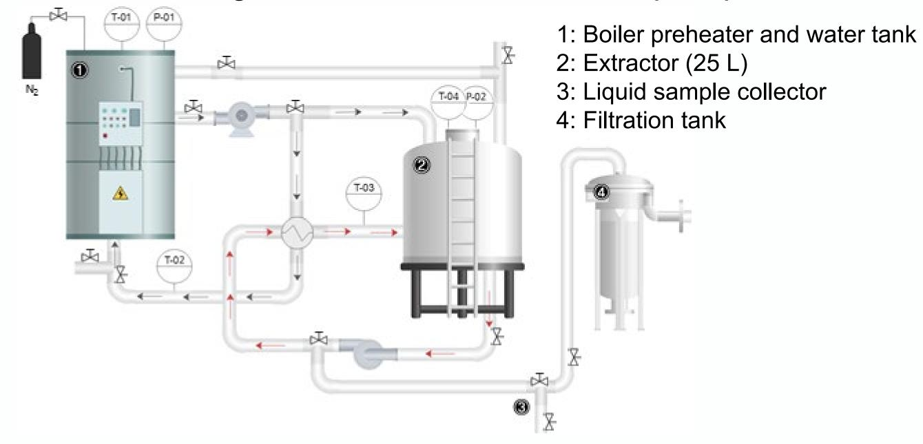
Experiments were carried out at 15 % biomass loading,  $181.1 \pm 0.6$  °C and a working pressure of 20 bar. The extraction/hydrolysis kinetics were followed.
