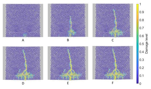
Fig. 4.16 Reinforced concrete beam damage development at different stages
