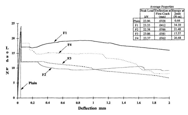
Fig. 2.12 Flexural load-deflections curves for plain concrete (PC), hooked end (F1), crimped (F2, F3) and twin cone (F4) fiber [174]
