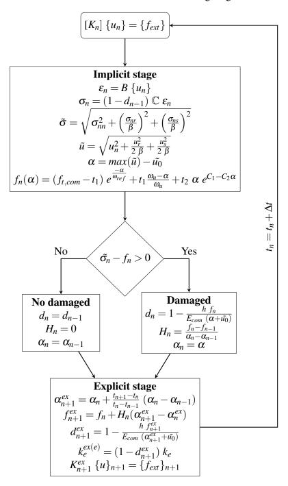
Fig. 4.3 Flowchart of the algorithm implemented for the interface element for fibers
