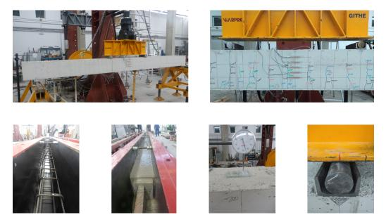
Fig. 7.14 Flexural beam set up
