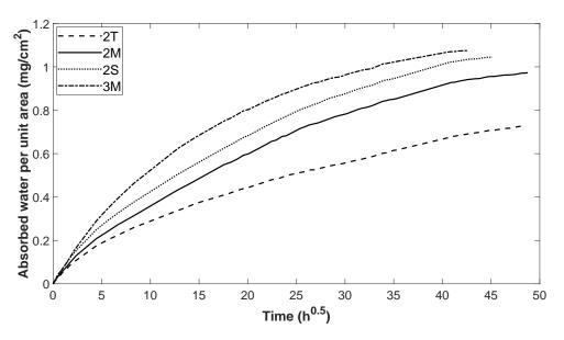
Fig. 6.14 Capillary suction curves for specimens
