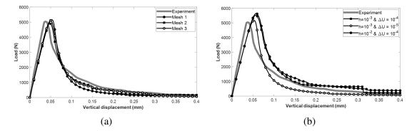
Fig. 4.8 Load/displacement curve obtained with (a) Different mesh (b) Different interface height and pseudo-step
