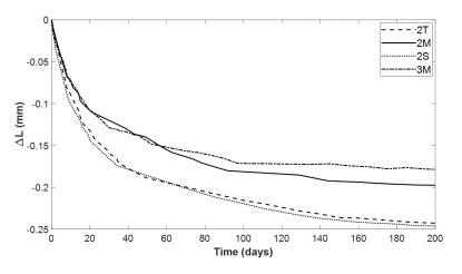
Fig. 5.15 Length change during shrinkage test
