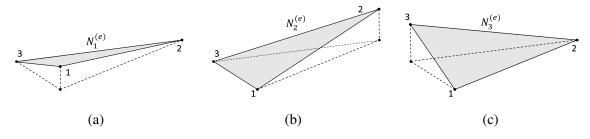
Fig. 3.7 Shape functions for linear triangle
