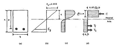
Fig. 2.9 Strain-stress distribution of SFRC beam [121]
