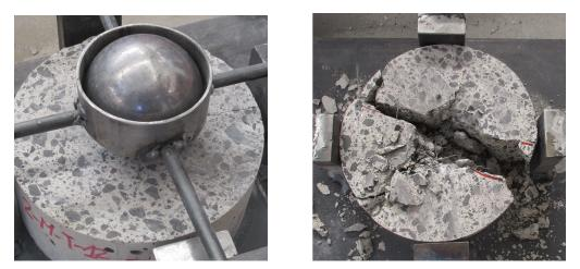
Fig. 5.12 Impact strength test
