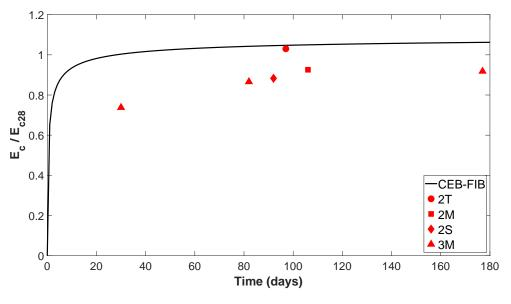
Fig. 6.1 Development of elastic modulus with time
