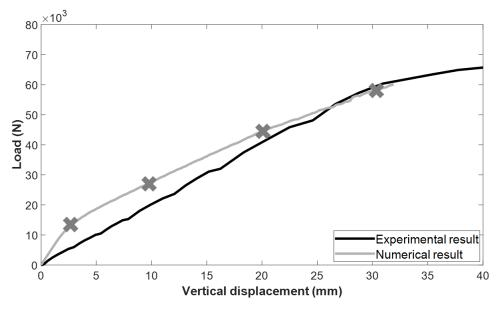
Fig. 7.29 Load/deflection curves of the beam made with the mix 3M
