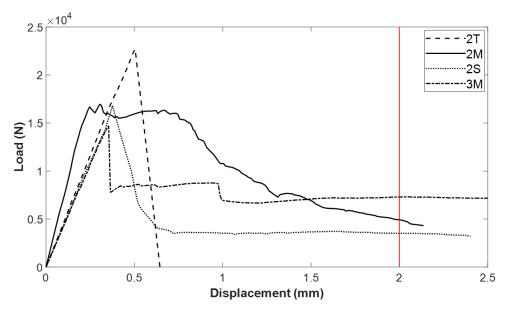
Fig. 6.8 Average load-deflection curves determined through flexural test
