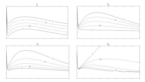
Fig. 3.14 Stress-crack opening displacement relation depending on  $t_1$ ,  $t_2$ ,  $c_1$ , and  $c_2$
