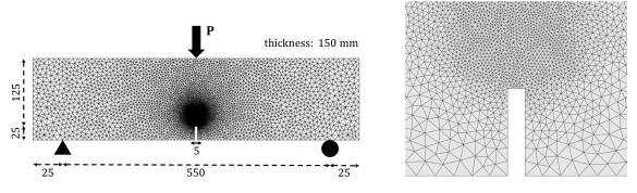
Fig. 7.2 Finite element model of tested notched beams
