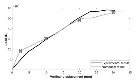
Fig. 7.19 Load/deflection curves of the beam made with the mix 2T
