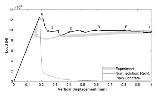
Fig. 4.13 Reinforced concrete beam load/displacement curve
