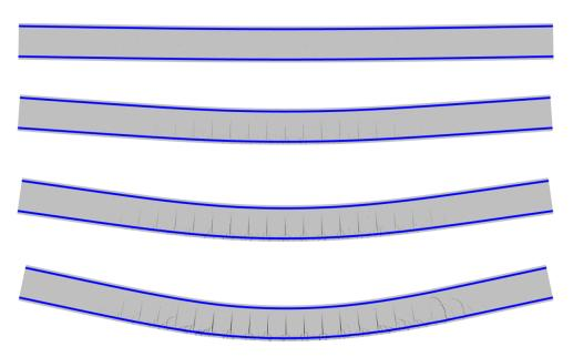
Fig. 7.28 Cracking of beams made with the mix 2S
