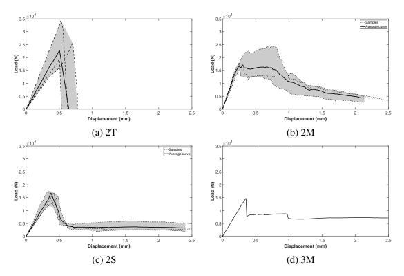
Fig. 5.7 Flexural test results of the different mixtures
