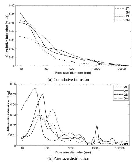
Fig. 6.13 Mercury intrusion porosimetry curves
