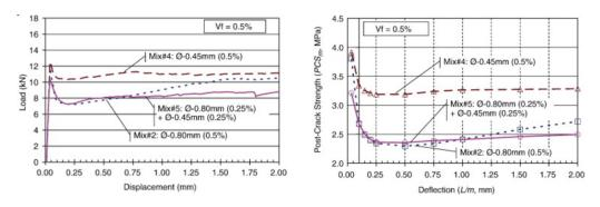
Fig. 2.2 Load-deflection curve and post-crack strength [19]
