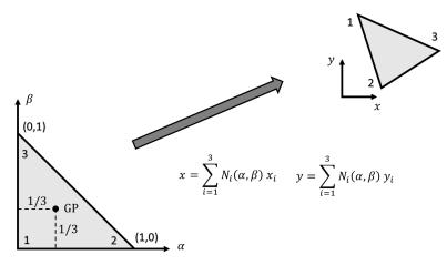
Fig. 3.8 Isoparametric mapping for linear triangle
