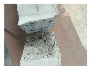
Fig. 6.5 Fibers crossing the cracking section
