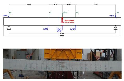
Fig. 7.16 Four-point bending beam tests
