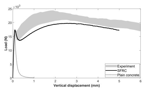
Fig. 4.11 SFRC beam Load/displacement curve
