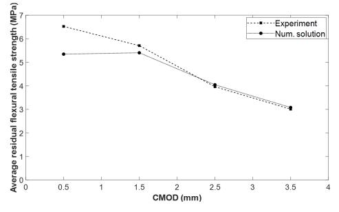
Fig. 7.8 Toughness index of numerical and experimental results
