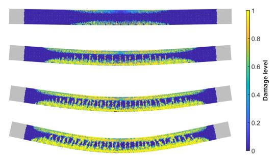
Fig. 7.24 Damage development in the beam made with the mix 2M
