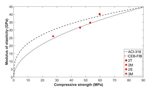
Fig. 6.2 Relationship between elastic modulus and compressive strength at 28 days
