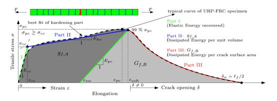
Fig. 2.6 Uniaxial tensile response of SFRC [194]
