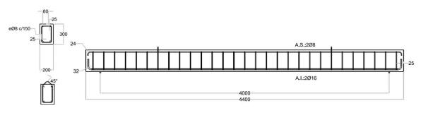
Fig. 7.15 Plans of the tested beams
