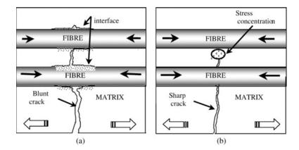
Fig. 2.10 Cracking appearance in presence of fibers: a) during static loading following a stage of fatigue loading, b) during static loading without previous fatigue loading [146]
