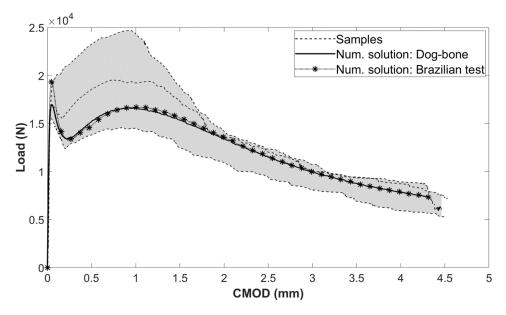
Fig. 7.7 Comparison of 2M notched beams modeled with tensile strength obtained through Dog-bone and Brazilian test
