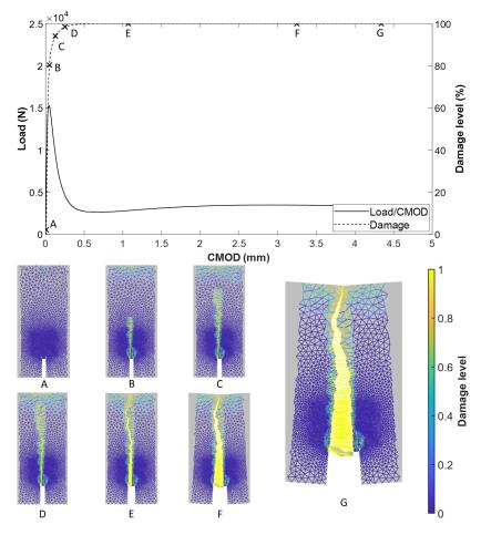
Fig. 7.11 Damage evolution of 2S notched beams
