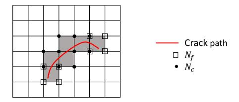
Fig. 3.2 Finite elements with discontinuities no aligned with a mesh
