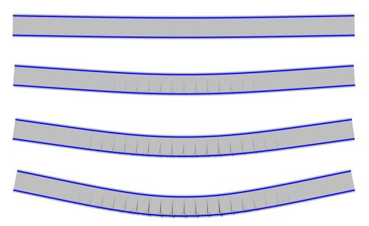
Fig. 7.22 Cracking of beams made with the mix 2T
