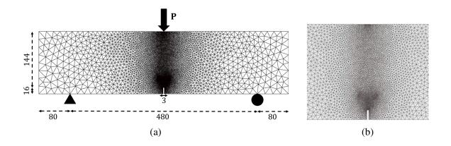
Fig. 4.7 Three point bending beam (a) Geometry and boundary conditions (b) Refined mesh
