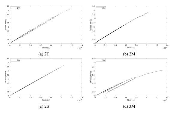
Fig. 6.4 Strain-stress curve of uniaxial tensile test
