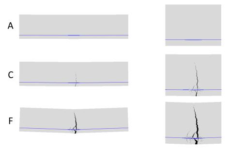
Fig. 4.14 Crack development at stages A, C and F
