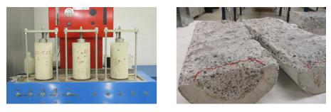
Fig. 5.10 Water penetration under pressure test set up and results
