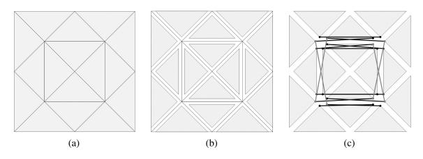
Fig. 4.4 Reinforcement discretization
