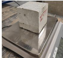
Fig. 5.13 Water absorption test
