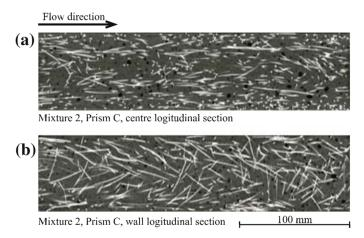
Fig. 2.4 Fiber orientation for different flow direction [166]
