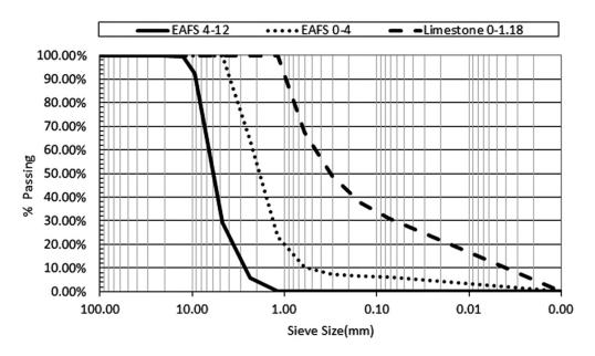
Fig. 5.1 Grading curves of aggregates
