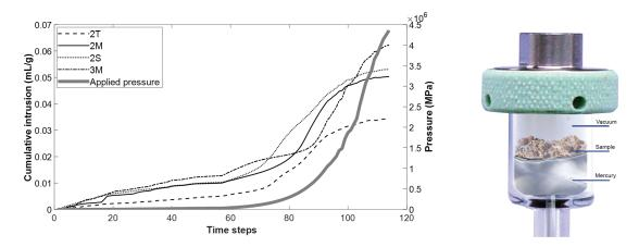
Fig. 5.11 Pressure and cumulative intrusion development during MIP test and the set up
