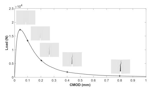
Fig. 7.4 Fracture development during the loading
