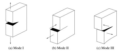
Fig. 3.1 Fracture modes for crack propagation
