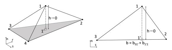
Fig. 3.4 3D and 2D interface element
