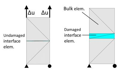
Fig. 3.3 Schematic diagram of interface elements model
