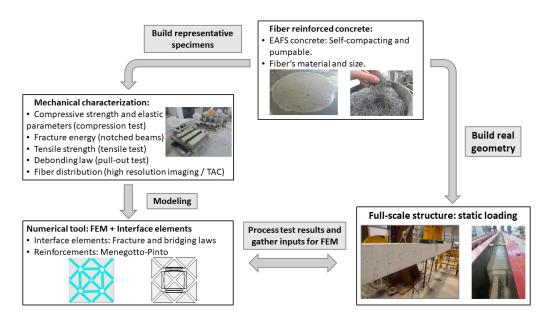
Fig. 7.1 Design methodology for steel fiber reinforced concrete made with EAFS
