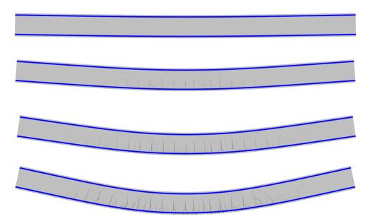
Fig. 7.31 Cracking of beams made with the mix 3M
