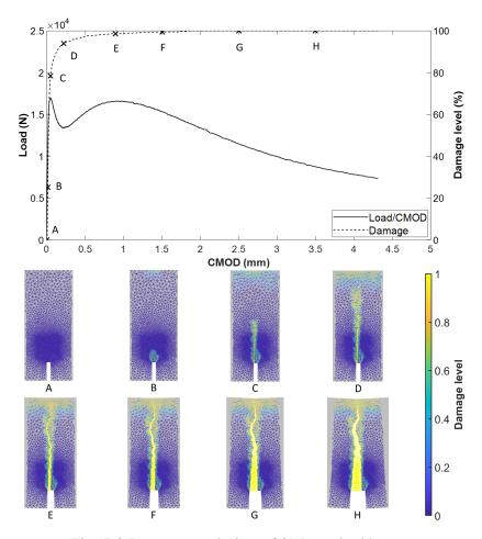
Fig. 7.9 Damage evolution of 2M notched beams
