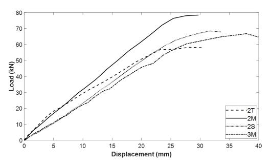
Fig. 7.17 Load/deflection curves of the beam
