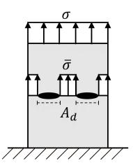
Fig. 3.10 Graphic representation of the damage
