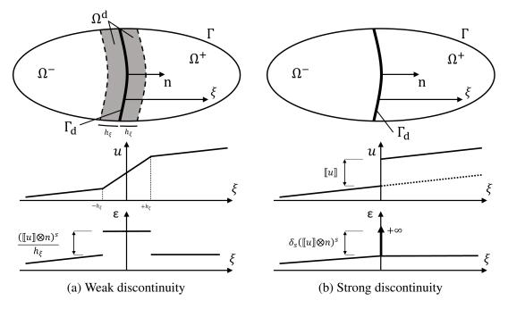
Fig. 3.9 Kinematic state of strong and weak discontinuity
