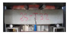
Fig. 5.6 Flexural test setup and failure
