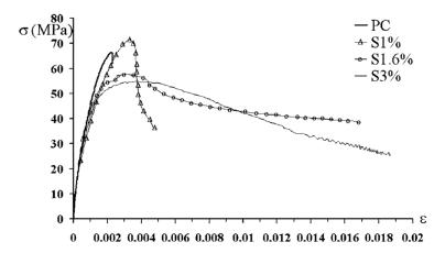
Fig. 2.7 Stress-strain curve for specimens without (PC) and with fibers (S1%, S1.6%, S3%) [31]
