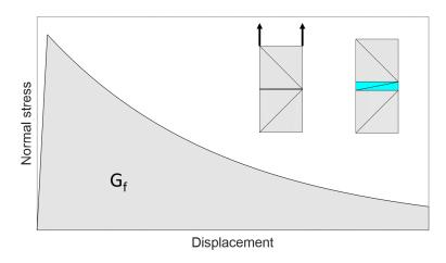
Fig. 3.12 Softening curve of a tensile damage model
