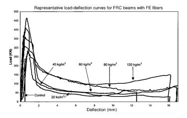
Fig. 2.8 Load-deflection curve in shear for fiber reinforced concrete [109]
