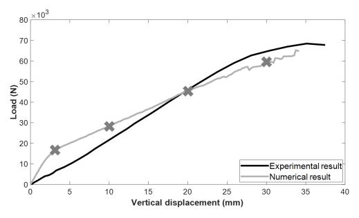
Fig. 7.26 Load/deflection curves of the beam made with the mix 2S
