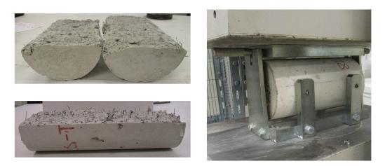
Fig. 5.4 Indirect tensile test
