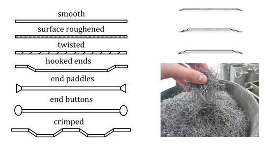
Fig. 2.3 Profiles of steel fibers used in concrete
