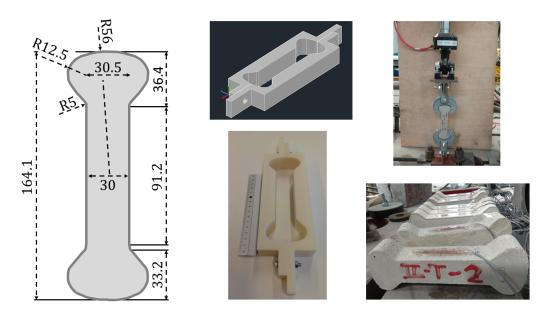
Fig. 5.5 Dog-bone design and set up
