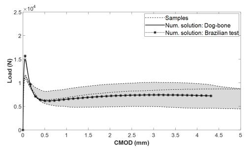
Fig. 7.12 Comparison of 3M notched beams modeled with tensile strength obtained through Dog-bone and Brazilian test
