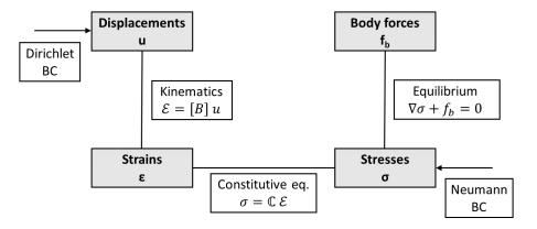
Fig. 3.5 Tonti's diagram of elasticity
