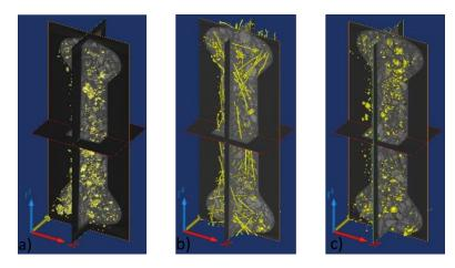
Fig. 6.7 XCT images for visualizing steel fibers and inclusions
