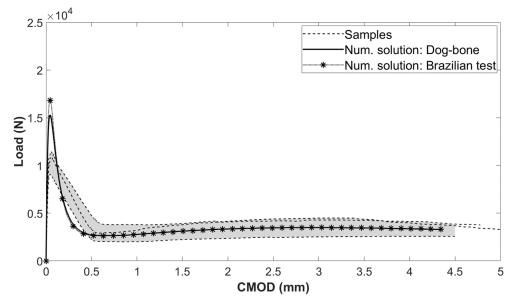
Fig. 7.10 Comparison of 2S notched beams modeled with tensile strength obtained through Dog-bone and Brazilian test
