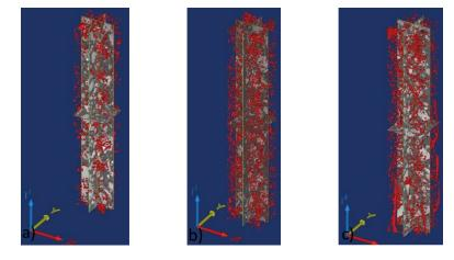
Fig. 6.6 XCT images for visualizing synthetic fibers and air voids
