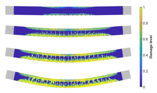
Fig. 7.30 Damage development in the beam made with the mix 3M
