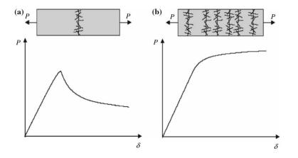
Fig. 2.5 Loading-deformation curve for post-cracking (a) softening and (b) hardening [47]
