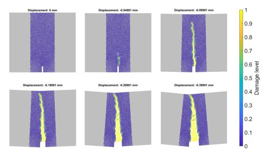
Fig. 4.9 Crack growth simulation and damage level of interface elements
