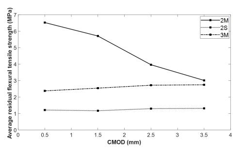
Fig. 6.11 Toughness index comparison
