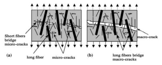
Fig. 2.1 Bridging effect of the fibers [129]
