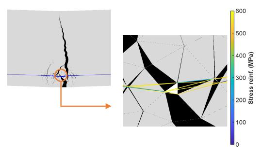
Fig. 4.15 Reinforcement bars discretization (Point F)
