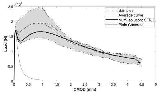
Fig. 7.6 Tested 2m notched beam Load/CMOD curve
