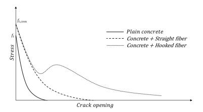
Fig. 3.13 Crack bridging curve for different fibers
