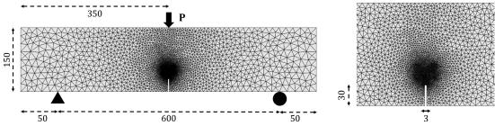
Fig. 4.10 SFRC beam geometry
