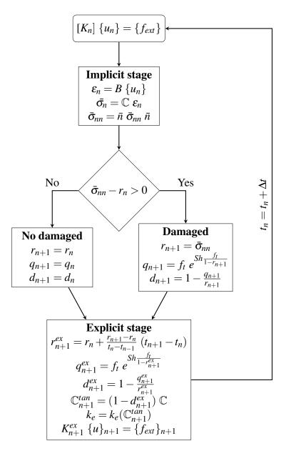
Fig. 4.2 Flowchart of the algorithm implemented for the interface element for plain concrete
