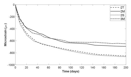
Fig. 6.15 Shrinkage strain results
