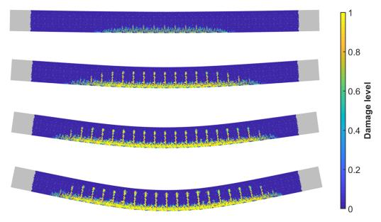
Fig. 7.21 Damage development in the beam made with the mix 2T
