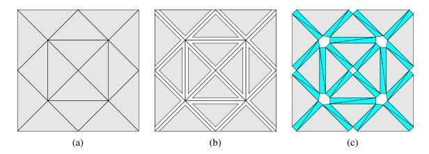
Fig. 4.1 Inserting interface elements into a standard mesh (a) Standard finite element mesh (b) Introduction of gaps (c) Insertion of interface finite element
