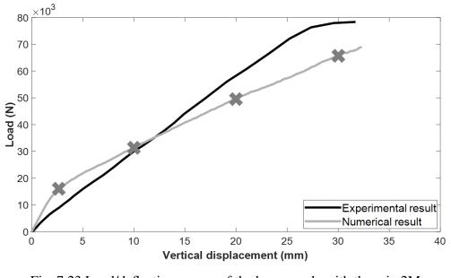
Fig. 7.23 Load/deflection curves of the beam made with the mix 2M
