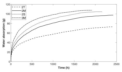
Fig. 5.14 Increase of mass during the capillary water absorption test
