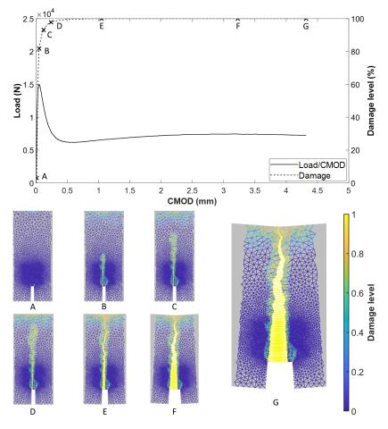
Fig. 7.13 Damage evolution of 3M notched beams
