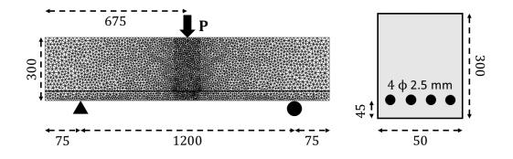
Fig. 4.12 Reinforced concrete geometry and cross section
