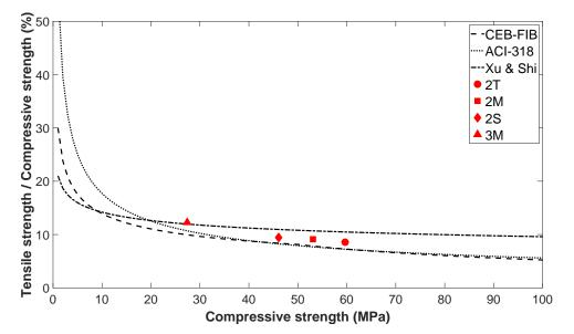
Fig. 6.3 Relationship between tensile strength and compressive strength
