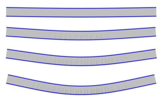
Fig. 7.25 Cracking of beams made with the mix 2M
