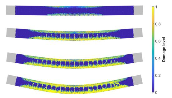
Fig. 7.27 Damage development in the beam made with the mix 2S
