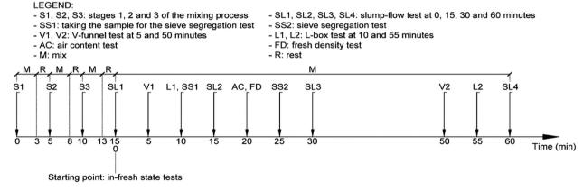
Fig. 2. In-fresh state testing program.
