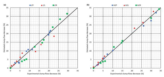
Fig. 6. Relationship between estimated and experimental slump flow: (a) CEM I; (b) CEM III/A.
