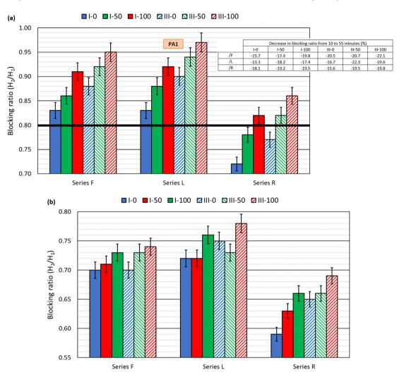
Fig. 9. Results of 2-bar L-box test: (a) at 10 min; (b) at 55 min.
