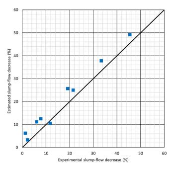
Fig. 7. Validation of the model developed with the data from other studies.
