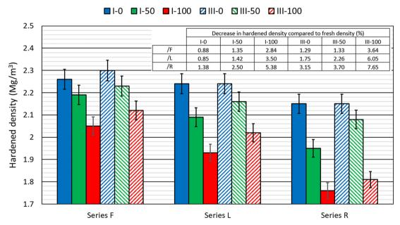
Fig. 14. Hardened density of the mixes and their lower real density in comparison with their fresh density.
