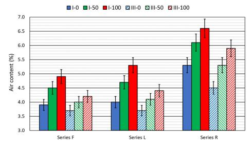
Fig. 11. Results of air content test.
