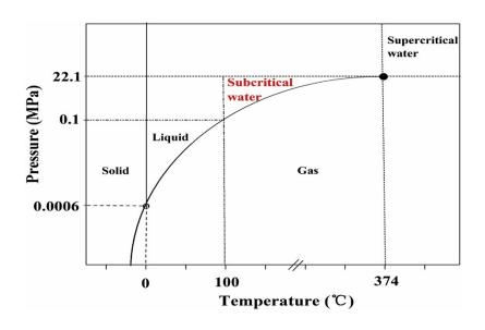
Water at temperature ranging from 100 °C (boiling point) to 374 °C (critical point); remains in a liquid state due to the application of pressure
