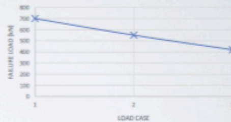
Influence of the fill height in the Failure Load
