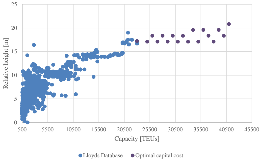
Figure 5. Relationship between the relative height and the capacity of container ships, with optimal alternatives selected according to capital cost.
