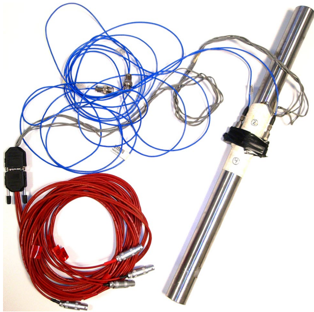
Fig. 14 Instrumented portion of the rod string with the strain gauges and the accelerometers
