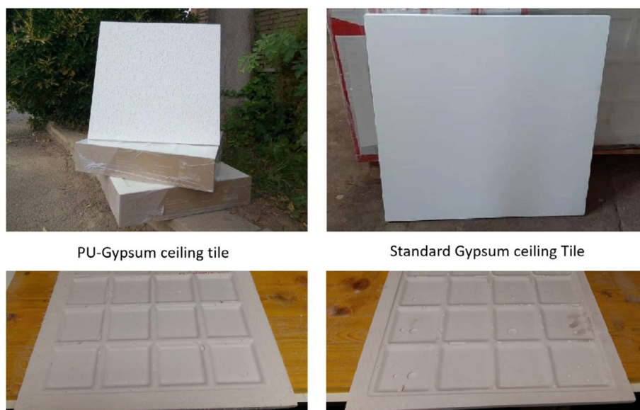
Fig. 1. Superficial appearance of the PU-Gypsum ceiling tile and Standard Gypsum ceiling tile.
