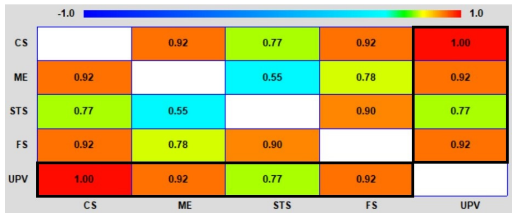
Figure 6. Spearman correlation matrix. Correlations between UPV readings and mechanical properties marked within the thick black border.
