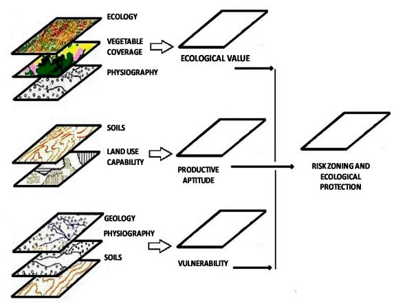
Figure 2. Superposition of the different georeferenced thematic layers worked with GIS interactively.
